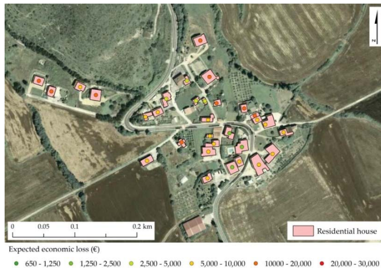
Figure 13. Close-up view of a residential house level wildfire risk map (eEL) for Marcalain (council cadaster polygon No. 8) expanded from Figure 12, over the June-2015 aerial photograph (idena.navarra.es). Other structures such as farm stores, churches and water deposits were excluded from the analysis. Overall, structures located in the periphery were more exposed to wildfires and presented higher potential losses. On the north side of rural communities, closer to shrublands and forest areas, higher wildfire hazard can enhance potential losses.
