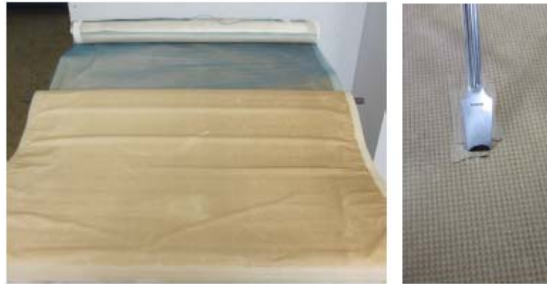
Figure 11-5: Unrolling of the membrane element showing the presence of a brown deposit on the membrane surface
