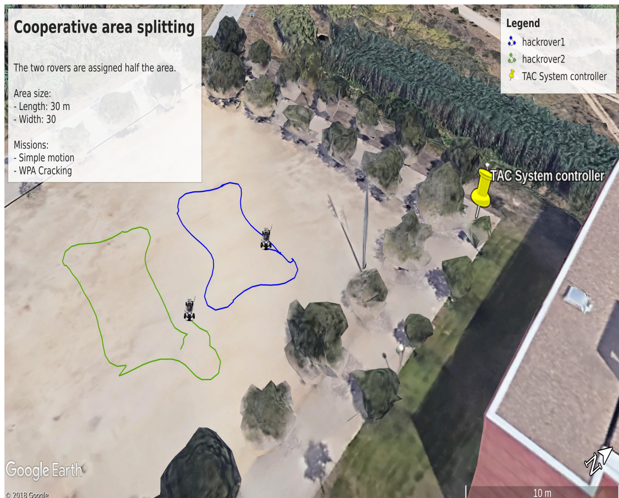
Figure V-29: Cooperative area splitting missions. The two rovers are assigned with half of the mission area. Missions with area splitting are: Simple motion and WPA cracking. Image created with Google Earth Google (n.d.) and TAC's mission data
