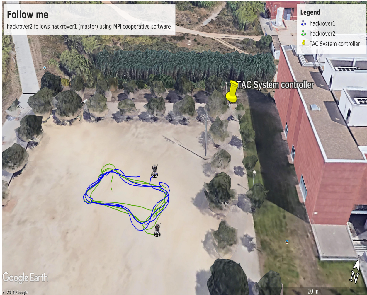
Figure V-30: Follow me mission. Hackrover2 follows hackrover1 using MPI collaborative software. Image created with Google Earth Google (n.d.) and TAC's mission data.
