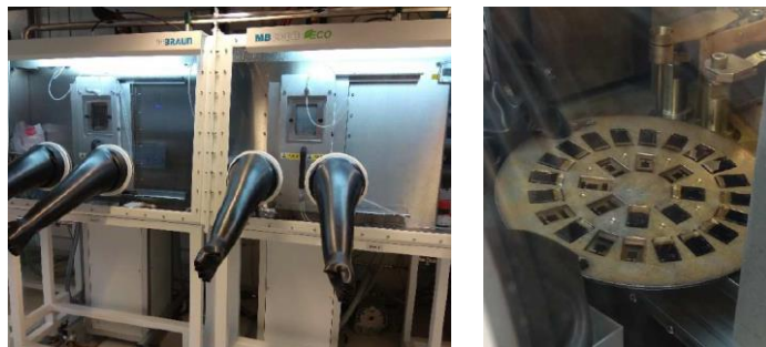
Figure 3.7: Picture of the outside of thermal evaporators (left) and the devices in the mask used for preparing PSCs devices at EPFL.
