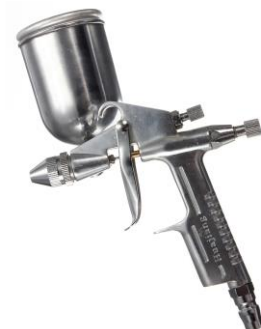
Figure 3.4: Spray pyrolysis gun used in the fabrication of the compact TiO 2 layer for PSCs.
