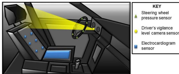
Figure 35: Smart vehicle sensors: steering wheel pressure sensor, camera, and electrocardiogram
