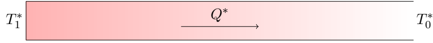
Figure 1.6: Conductive heat flux Q^* through a semi-infinite bar, induced by a temperature difference T_1^* - T_0^* .
