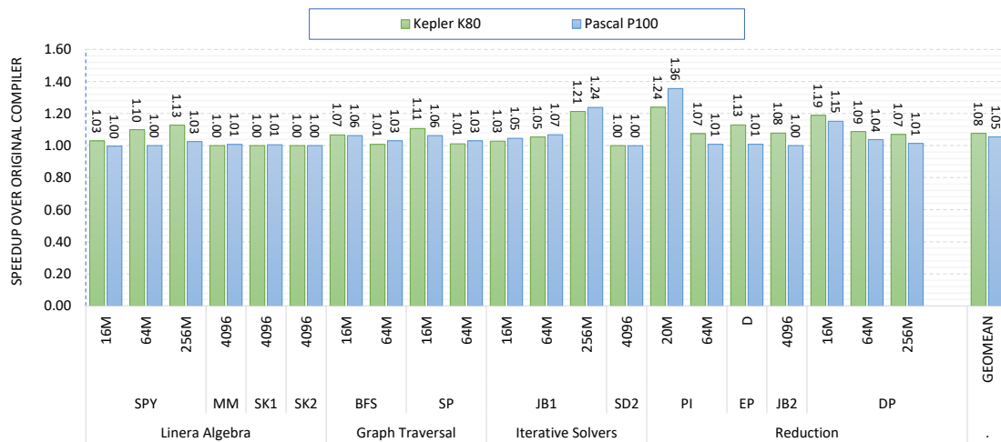
Figure 6.7: Application based speed-up of optimized dynamic scheduling over static cyclic scheduling.
