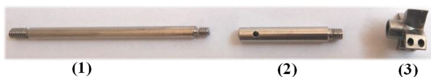
Figure 9.4. Picture of the gas entrainment impeller in its three different parts
