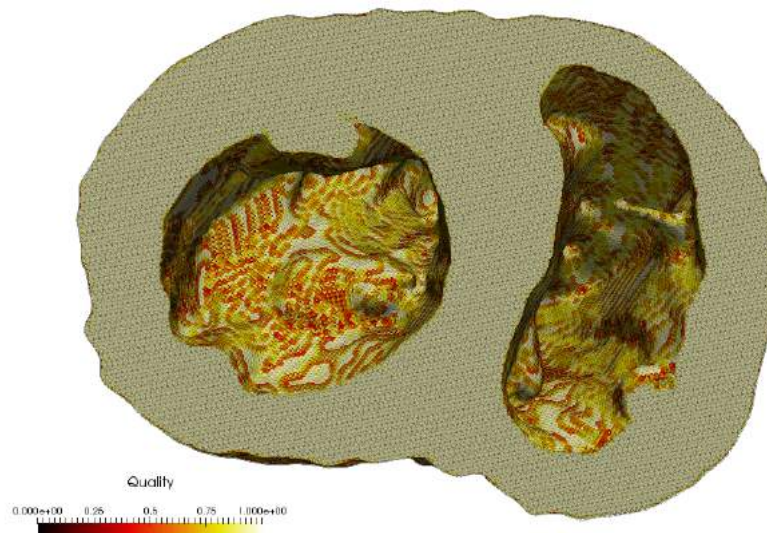
Figure 6.4: Geometry discretization. Element shape quality analysis of the control case mesh.
