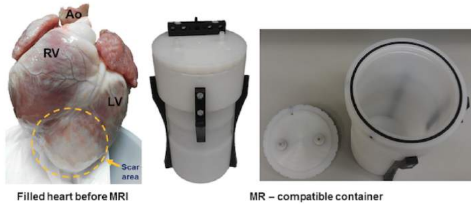
Figure 2.5: Cardiac Magnetic Resonance ( ex vivo ). Explanted heart filled and the container Magnetic Resonance compatible . Figure from [31].
