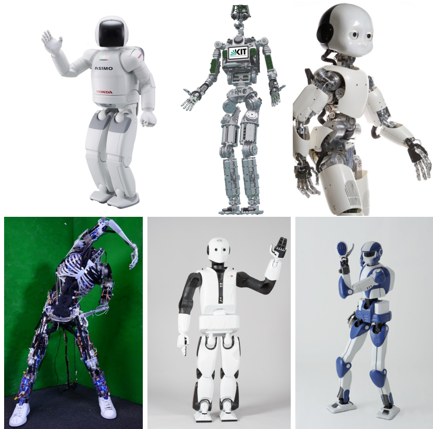
Figure 1.1: Some state of the art full-size humanoid robots. Upper row: ASIMO [Sakagami and Watanabe, 2002], ARMAR-4 [Asfour et al., 2013] and iCub [Metta et al., 2008]. Lower row: Kenshiro [Nakanishi et al., 2012], REEM-C [Tellez et al., 2008] and HRP-4 [Kaneko et al., 2011]
