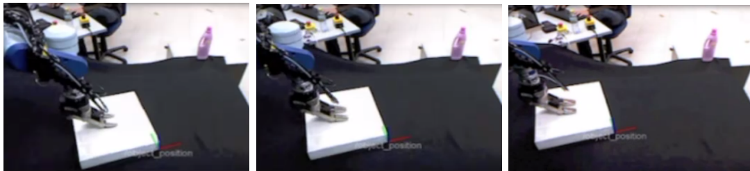
Figure 5.5: Object sliding experiment. The robot slides the box from the starting position (left) to the target position (right). The object pose is acquired by a model based tracker and depicted as a reference frame.
