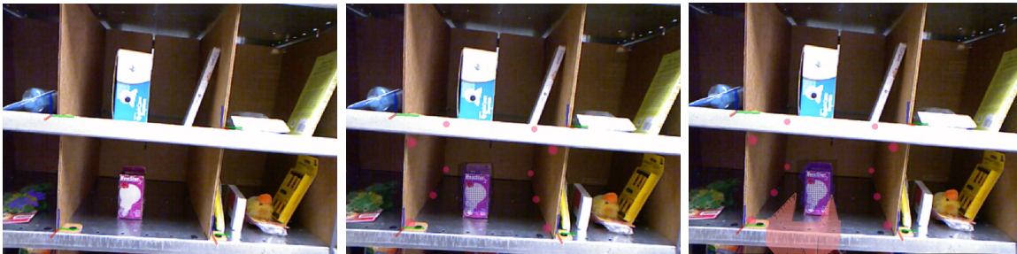
Figure 6.11: Grasp planning process for the APC challenge. Left: Initial image with bin reference frame. Middle: object segmentation, clustering and recognition. Right: grasp planning.
