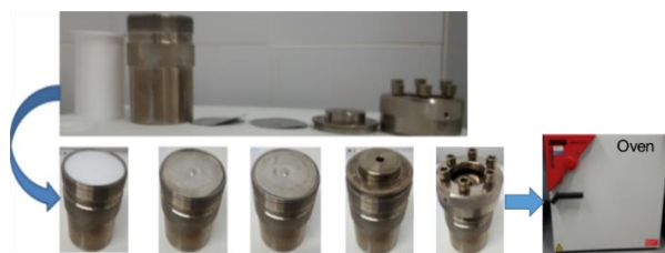
Figure 2.1: The mounting steps for the autoclave vessel ready to be introduced in the oven.
