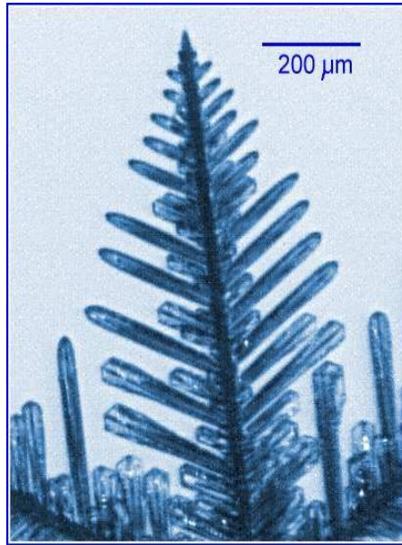
Figure 1.3: Dendritic growth and formation of sidebranches in a needle-crystal structure (Courtesy of Prof. Ken Libbrecht, Physics Dept., Caltech, Pasadena, USA).
