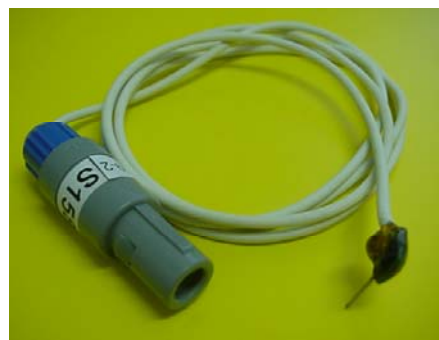
Figure D. 3. Details of probe packaging and wiring.
