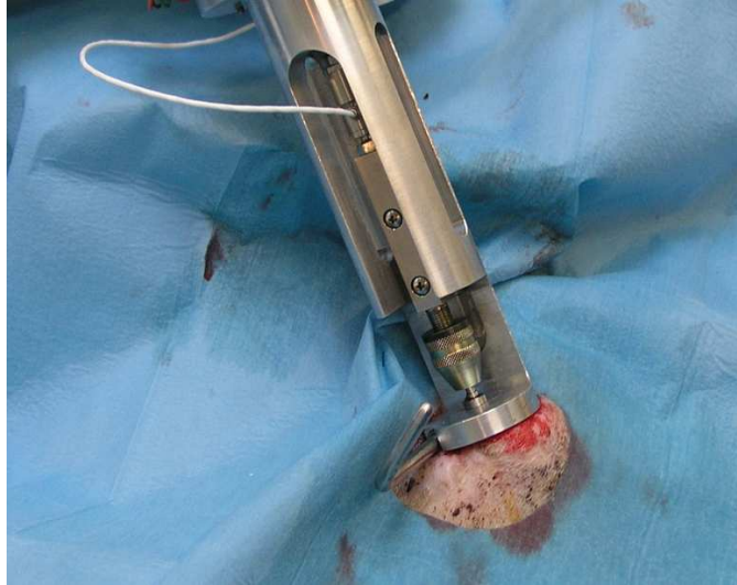
Figure 6.31: For the in vivo compression of implanted scaffolds, the developed compression device was connected to the piston from the exterior.
