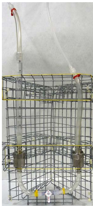
Figure 3.36: Setup for measurement of transported volume per half-cycle. Left side of the tubing was replaced by a 10 ml polystyrene pipette section.
