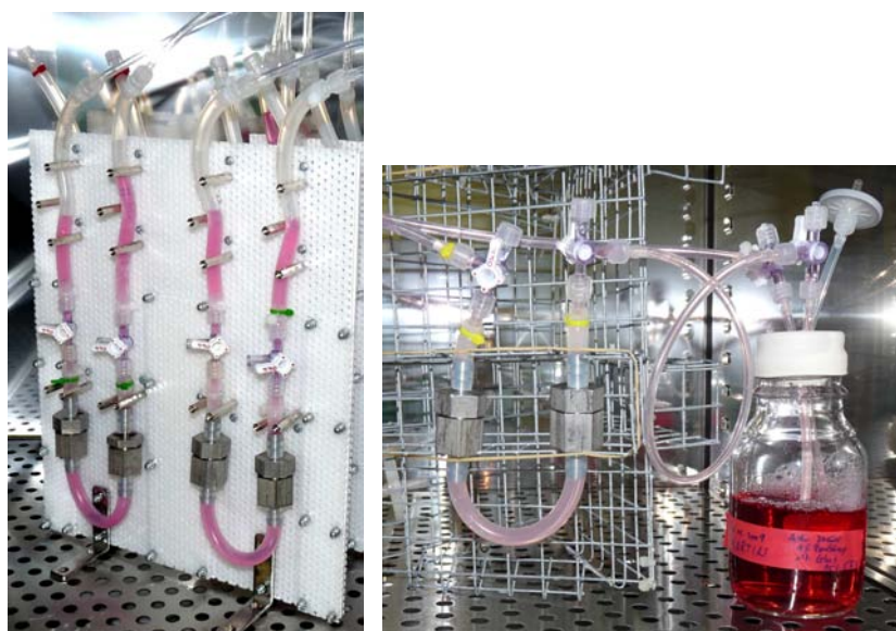
(a) Cell seeding phase including tubing for cell suspension level oscillation. (b) Cell culture phase including the medium reservoir.
