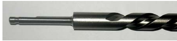
Figure 6.3: The shank of a commercial 11 mm HSS burr was modified to fit into a surgical drill.
