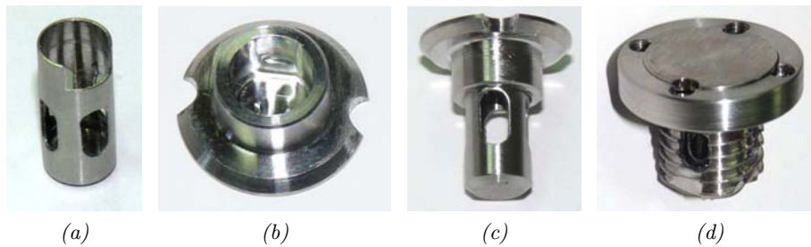
Figure 6.8: Alignment of the apertures for tissue ingrowth. The internal cage (a) had a profile on its top which corresponded to the profile in the cap (b). The cap and internal cage (c) was then inserted into the external cage. The cap notches aligned with the holes did ensure the alignment of the apertures (d).
