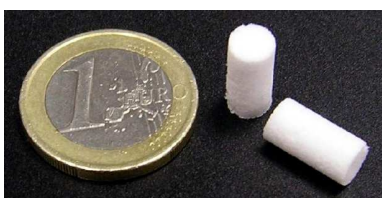
Figure 2.2: PLA/glass scaffolds used for the material characterization and later cell culture.
