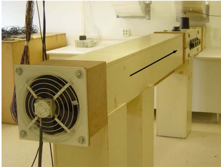
Figure 3.1: Tube and input noise source (fan)
