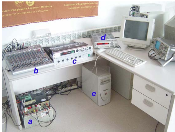
Figure 3.3: Signal-processing instrumentation composed by (a) DSpace system, (b) mixing console, (c) audio amplifier, (d) signal generator, (e) host PC, plus the oscilloscope
