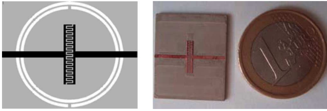
Fig. 3. Layout and photograph (top face) of the fabricated device. Dimensions are: line width W = 0.8 mm, external radius of the outer ring r = 7.3 mm, rings width c = 0.4 mm and rings separation d = 0.2 mm; the interdigital capacitor, formed by 28 fingers separated 0.16 mm, has been used to achieve the required capacitance value.
