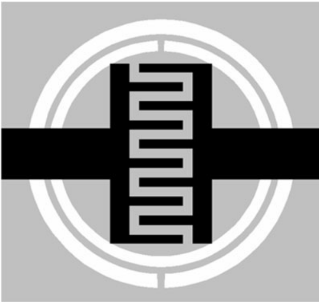
Figure 3 Unit cell of the balanced CSRR-based CRLH transmission line used for the design of the UWB band pass filter. The considered substrate is the Rogers RO3010 with thickness h = 635 \mu\text{m} and dielectric constant \epsilon_r = 10.2 . Dimensions are as follows (in reference to Fig. 1): r_{\text{ext}} = 2.10 \text{ mm} , d = 0.11 \text{ mm} , c = 0.22 \text{ mm} , and c = 0.16 \text{ mm} for the external and internal ring, respectively; the width of the host line is W = 0.80 \text{ mm} and the capacitor is formed by five face-to-face fingers separated a distance of 0.16 \text{ mm} (finger length and width are 0.84 and 0.14 \text{ mm} , respectively)
