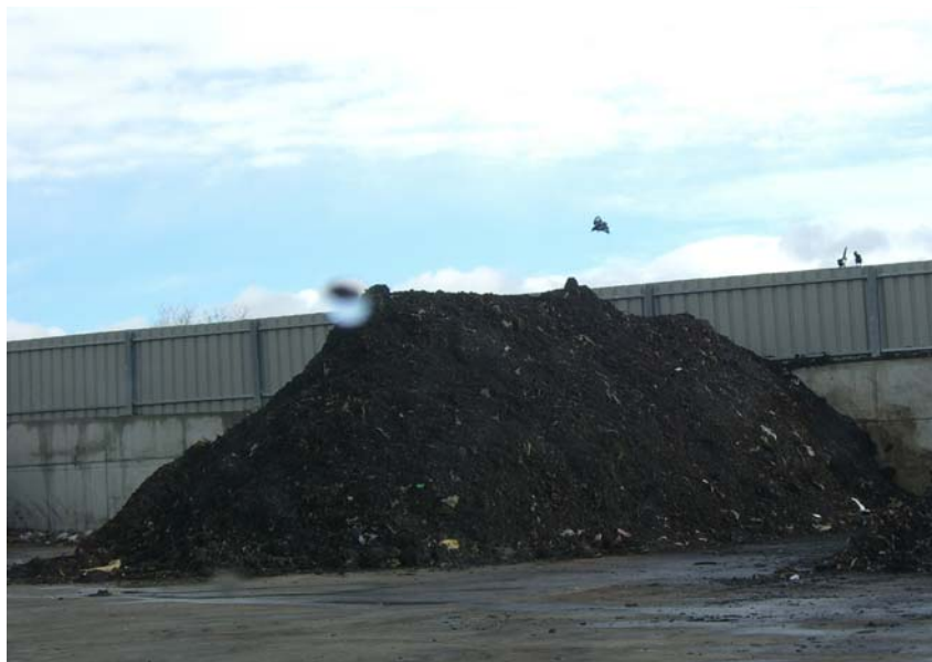
Figure 5.4. Appearance of a windrow in the maturation area.
