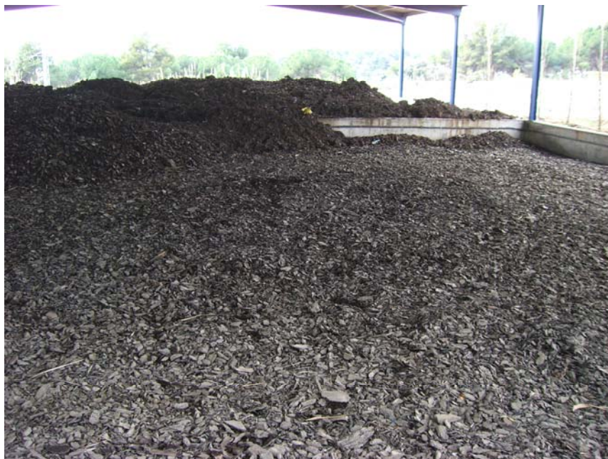
Figure 7.5. Detail of Biofilter 3 (first day of analysis) at the anaerobic digestion plus composting plant.
