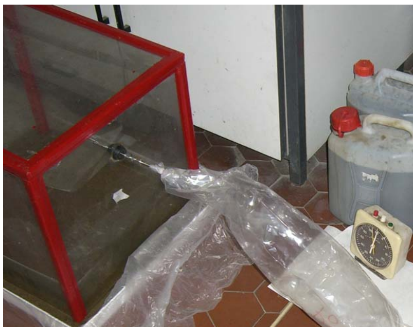
Figure 8.3. Gaseous samples collection in the static chamber. A Nalophane bag was connected and filled at the output port at a flow rate of 0.35 \text{ m}^3/\text{h} .
