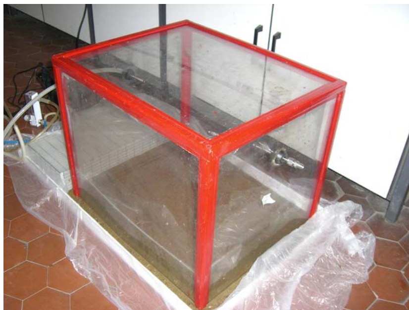
Figure 8.2. Static chamber (Plexiglas® material) used to sample gaseous emissions from the anaerobic digestion plant.
