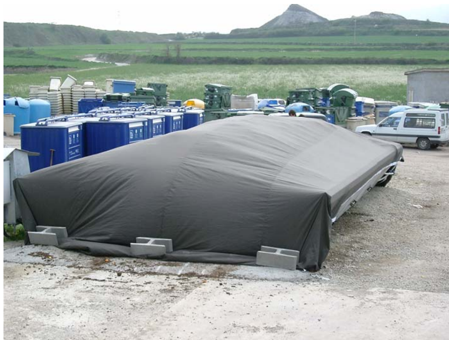
Figure 5.3. Confined windrow module with the textile liner cover.
