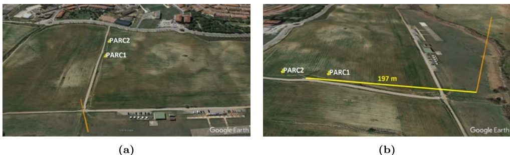
Figure 6.18: Images of the scenario taken from Google Earth with the vertical flight path information. Ascending velocity of 2 m/s. (a) North-west orientation. (b) South-west orientation.
