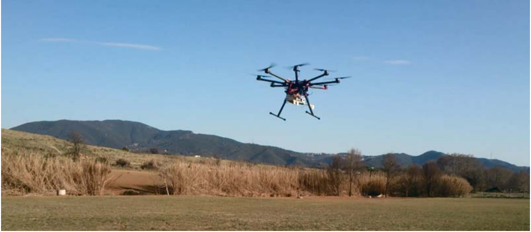
Figure 6.2: Fully polarimetric ARBRES-X SAR integrated in the UAV MP and flying in the RACBSA airfield during a measurement campaign.
