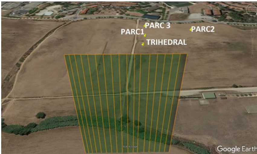
Figure 6.11: Disposition of the calibrators in the scenario and flight path performed by the UAV MP. Image from Google Earth.
