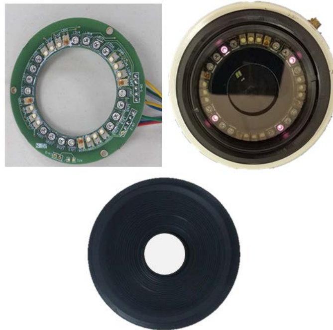
Figure 3.12 PCB with the LED ring and view of the LED ring mounted inside the cylinder (top) and view of the inside of the front conus (bottom).
