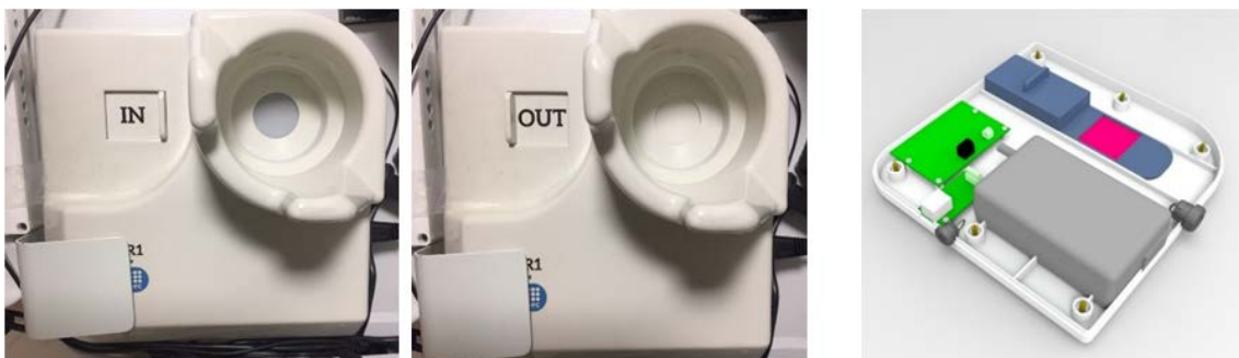
Figure 3.15 standard calibrated sample in the “IN” and “OUT” positions (left); and design of the interior of the base where the power supply, electronic boards, standard calibrated sample and other parts of the system are located (right).
