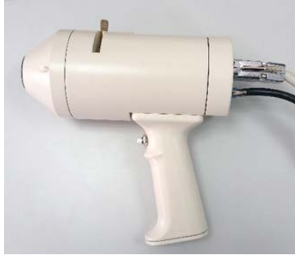
Figure 3.10 Overview of the multispectral head including the cylinder and the conus.
