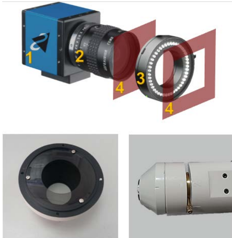
Figure 3.13 Distribution of the multispectral head components (top): (1) camera, (2) objective lens, (3) LED ring, (4) polarizers; Polarizer attached to the conus (bottom left) and top view of the multispectral head with the lever allowing the degree of polarization to be changed (bottom right).
