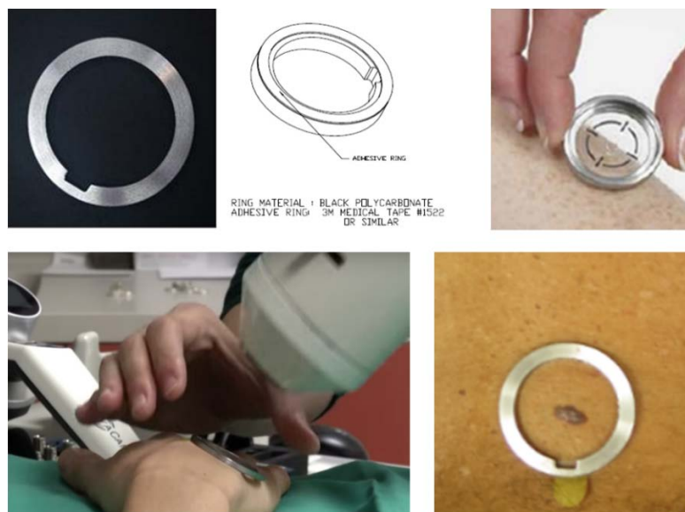
Figure 3.8 Big metal ring for the acquisition of the 3D, OFI and multispectral system (top left), small metal ring for the confocal microscopy acquisition (top right), and the big metal ring being used at the clinical setting (bottom).
