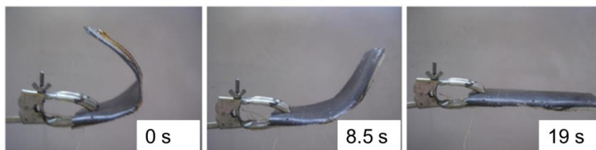
Figure I-19. Morphing wing made of a styrene-based shape-memory thermoset by Yu et al. [145] .
