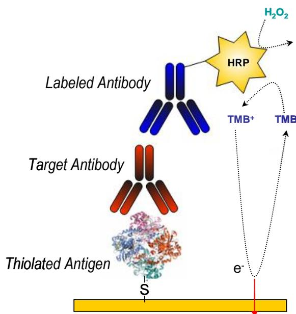
Scheme 3.2. Architecture of the immunoassay including electrochemical detection
