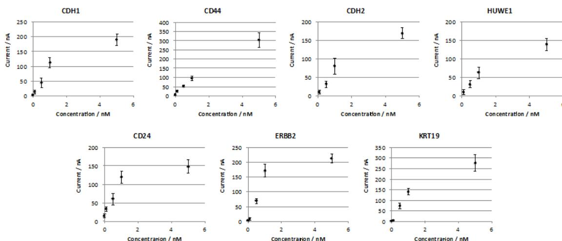
Figure 4.8 (SI). Calibration curve for each of the seven amplicons selected for the preparation of the low-density electrochemical sensor arrays (n=8).
