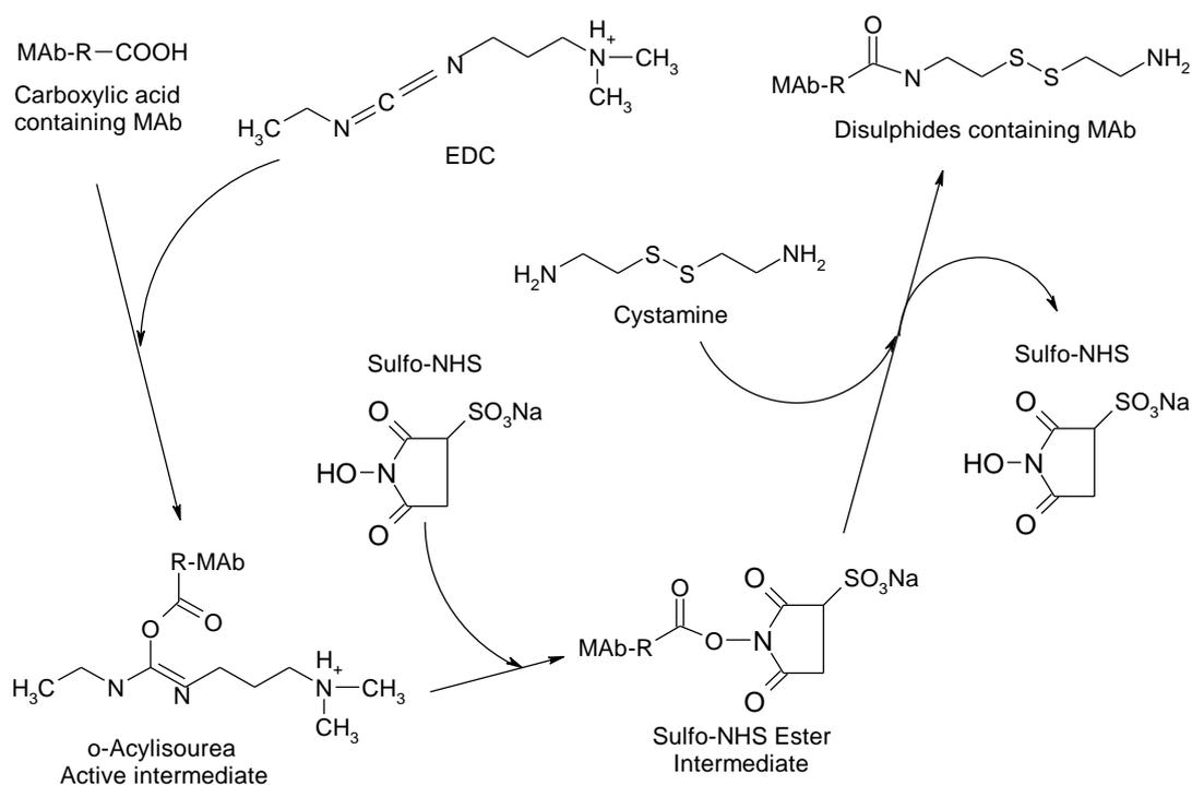
**Figure 1.8. Reaction scheme of the introduction of disulphides via -COOH residues.**
