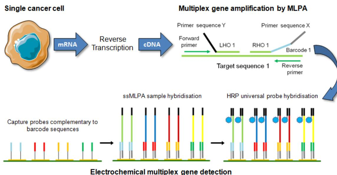
Figure 1.11. Schematic representation of the simultaneous barcode-based electrochemical detection of multiple breast cancer related mRNA markers from a single tumour cell using RT-MLPA.
