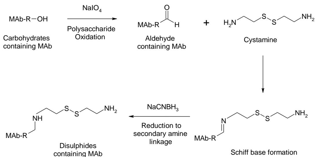
**Figure 1.9.** Reaction scheme of the introduction of disulphides via carbohydrates.
