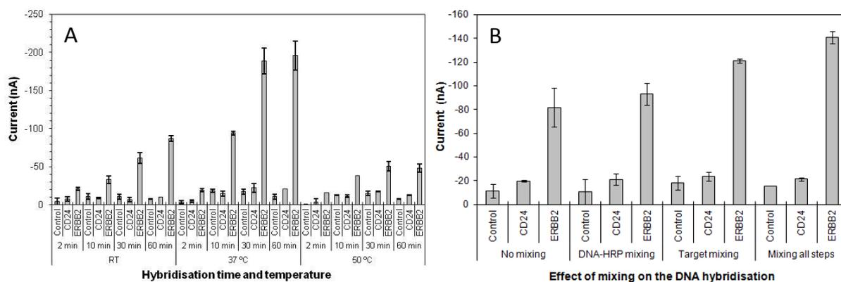
**Figure 4.5.** Effect of time, temperature (A) and mixing (B) on the DNA hybridization efficiency of the synthetic ERBB2 amplicon.
