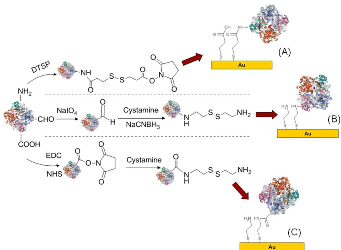
**Scheme 3.1.** Reaction schemes for the disulphide modification of the antigen protein through the different moieties (A) amine, (B) carbohydrates and (C) carboxyl groups.
