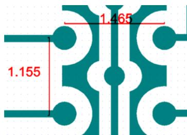
Figure 4.7 (SI). CAD of the 64-electrode array (dimensions in mm)
