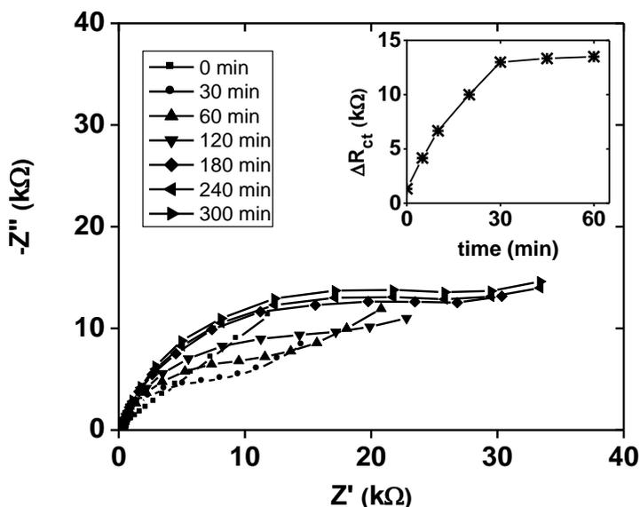
Figure 2.5. Complex impedance plot (in 1 mM  $K_3Fe(CN)_6$  solution in PBS pH 7.4) for the formation of a SAM of NSE21-CHO at gold electrodes at different exposure times. Inset: Impedance variations for the specific interaction of NSE with NSE21-CHO modified surface.
