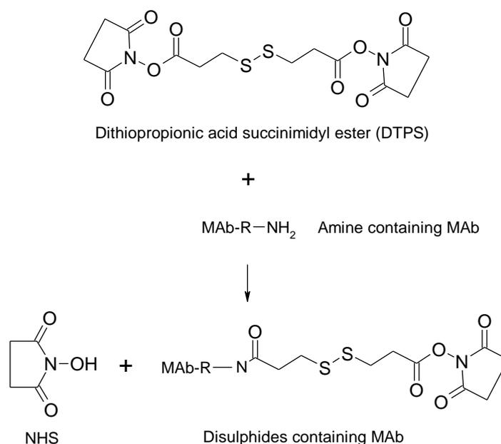
Figure 1.7. Reaction scheme of the introduction of disulphides via  $-NH_2$  residues.
