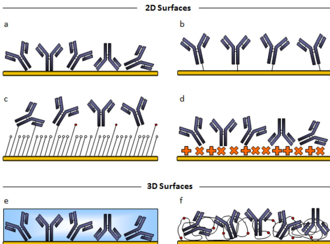
**Figure 1.6.** Schematic representation of different antibody immobilisation approaches: a) physisorption of unmodified Abs, b) chemisorption of chemically modified Abs, c) covalent immobilisation through a SAM, d) bioaffinity-based immobilisation, e) physical entrapment and f) covalent immobilisation on a matrix containing reactive groups.
