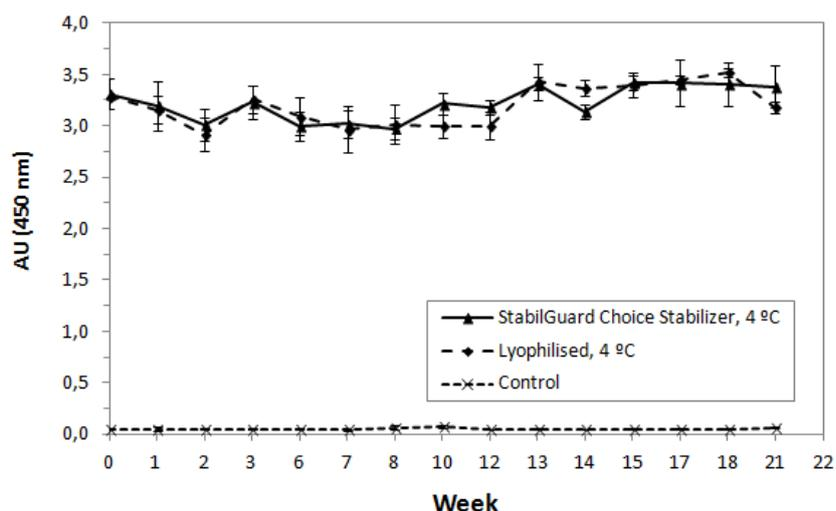
Figure 5.5. Absorbance signals for the HRP-labelled DNA (10 nM solution) binding levels for different storage conditions: i) prepared in StabilGuard® Choice commercial stabilizer and stored 4 °C and ii) lyophilized, stored at 4 °C and reconstituted in TBS containing 1 M NaCl (n =3).
