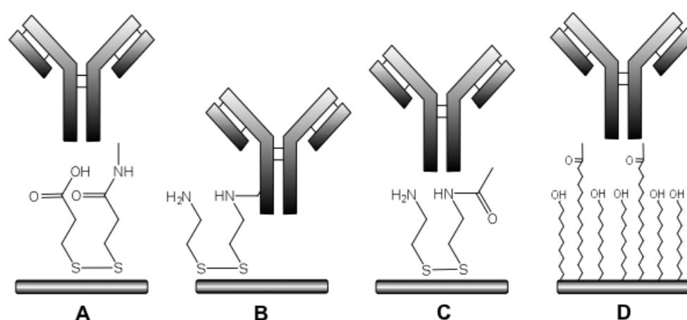
**Scheme 2.1.** Functionalization strategies of bare gold substrates via direct bio-SAM using disulphide-containing antibody chemically modified via their primary amines (A), carbohydrates (B) and carboxylic acids (C) and via classic SAM (D) using unmodified antibodies attached on a long-chain of alkanethiols previously self-assembled onto a bare gold substrate.
