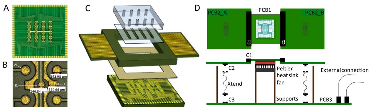
**Figure 4.1. Electrochemical detection platform. A) 64-electrode array realised on PCB; B) Magnified image of the PCB chip showing the working (W), counter (C) and reference (R) electrodes; C) Schematic representation of the sensor (1. PCB chip, 2. Anisotropic conductive adhesive tape, 3. PCB carrier, 4. Microfluidic channels of double-sided adhesive tape and 5. Laser machined PMMA gasket); D) Detection unit fully assembled.**
