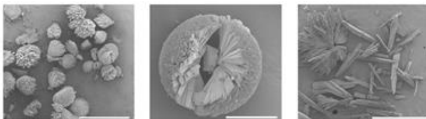
Figure 17 SEM images of RS . The images reveal the octahedral morphology of the R and S crystals, and the intergrown, needle-shaped crystals of RS , and confirm that all the MOFs are homogeneous. Scale bars: 1 mm (left); 50 \mu\text{m} (middle); and 500 \mu\text{m} (right)
