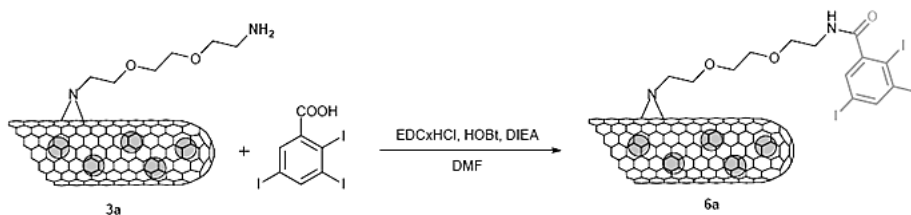
Figure 3.34 Tagging of the amino groups of SmCl 3 @SWCNTs-NH 2 ( 3a ) with the 2,3,4-triiodophenyl motif.
