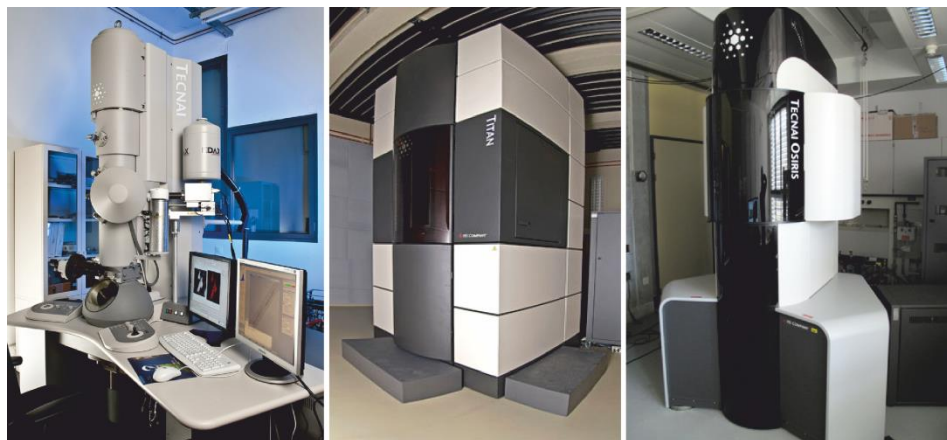
Figure 2.6 TEM microscopes used for research focused on functional carbon nanotubes in this thesis. From left to right: FEI's Tecnai G2 F20 (ICN2, Bellaterra, Spain), FEI's (QU-Ant EM) Titan (EMAT, Antwerpen, Belgium) and FEI's Tecnai OSIRIS (EMAT, Antwerpen, Belgium). All of them equipped with EDX and EELS spectrometers.
