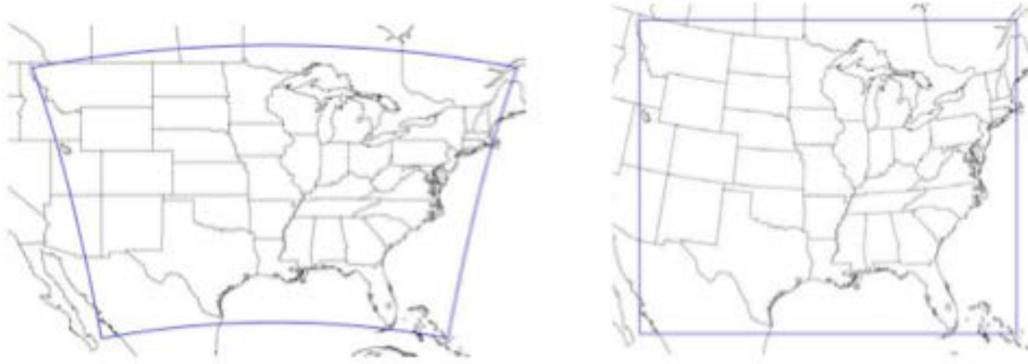
Figure 7. Horizontal coordinate system in NMMB for a domain centered at 38N, 92W. On the left side: domain plotted on a regular latitude longitude map background. On the right: the same domain is projected on a rotated latitude longitude map background (extracted from Janjic and Gall, 2012).
