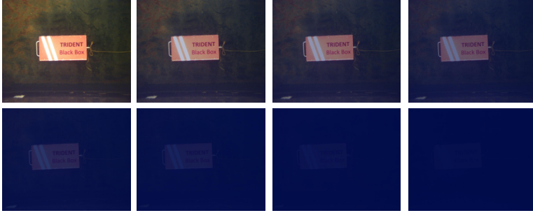
Figura 5.8: From left to right top to bottom, tracking algorithm scenario in decreasing HIL visibility scenario.
