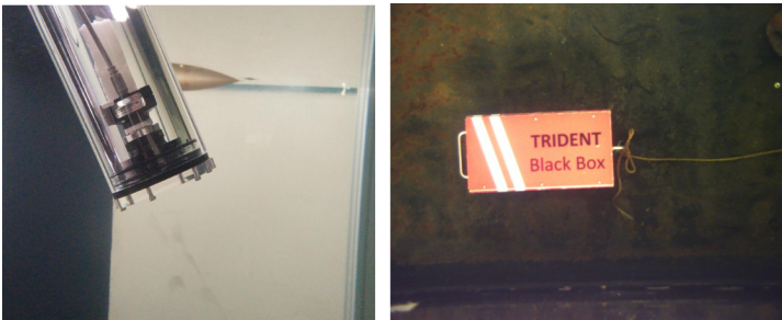
Figura 5.7: Image acquisition setup. Left: camera in a cylinder moving in the water surface. Right: black box mock-up captured from the camera.
