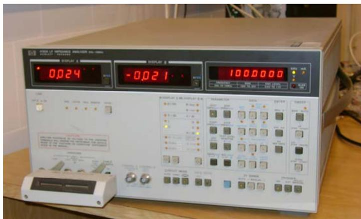
Fig. B.3 Four-point equipment (top) and a 4192A LF impedance analyzer (bottom).
