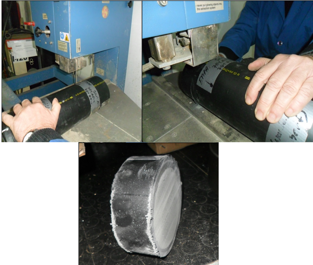
Figure 2-22. Pre-cutting a slice of the core sample under dry conditions with a band saw.
