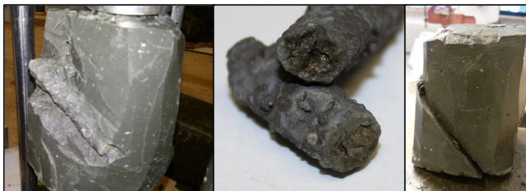
Figure 2-12. Failed samples due to the breakage during the preparation.
