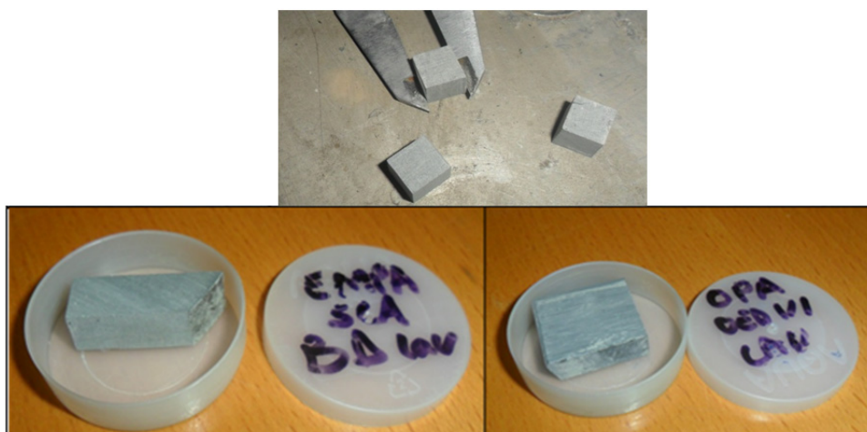
Figure 2-25. Samples for MIP and psychrometer tests cut under dry conditions with a band saw.
