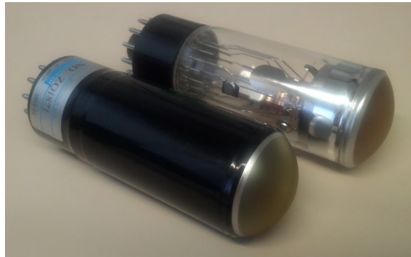
Figure 1.8.: Photomultiplier tube selected for the CTA consortium. The right one, shows the dynodes structure and the left one is covered by mu-metal foil.
