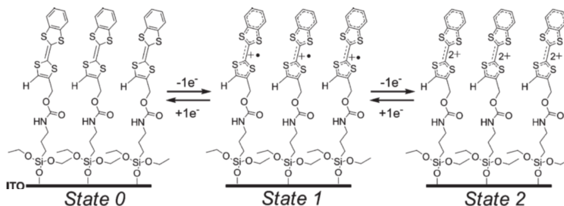
Figure 5.8. Schematic representation of the electrochemical activity of TTF-triethoxysilane derivatives on ITO surface.
