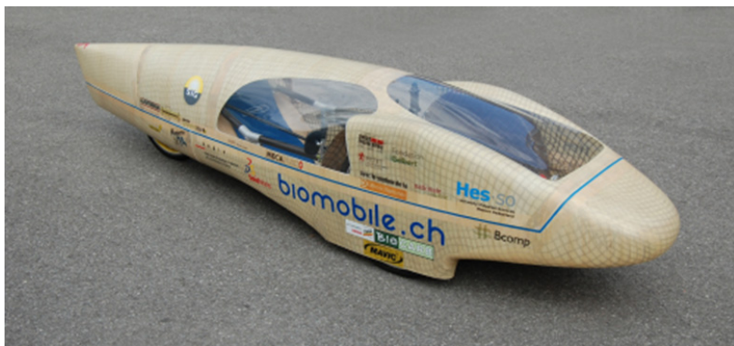
Figure 1. Prototype vehicle, “verte”. Lower part of the body frame made of fully bio-based composites [M. Perraudin, BioMobile.ch].
