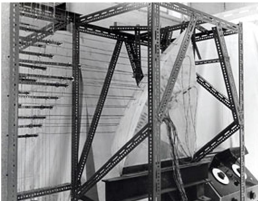
Fig. 3-2-58: Model C being subjected to loads representing wind forces (c.1958). Photo: © Peter Morice
