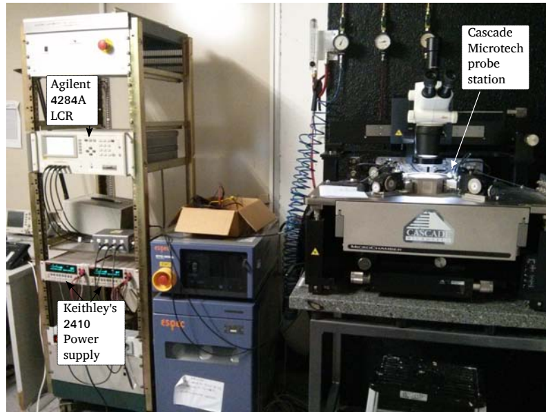
Figure 2.9: CNM characterization lab. The Cascade probe station is on the right side of the picture and the two power supplies are on the left.
