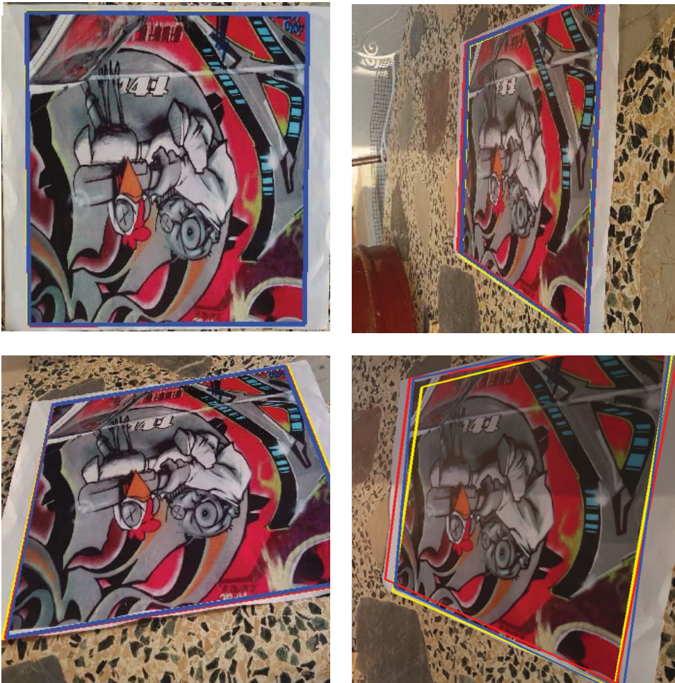
Figure 4.19: Experiments with real images of a planar object. In these images the results provided by the EPPnP (red rectangle), the OPnP (yellow rectangle) and the CEPPnP (blue rectangle) are shown.
