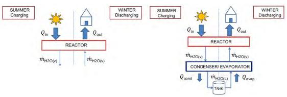
Figure 10. Open (left) vs. closed (right) systems with integrated reactor [49].
