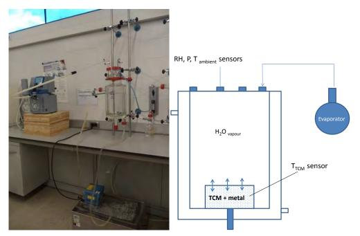
Figure 14. Self-developed setup to test TCM corrosion for closed configuration systems. Left: general view, right: scheme of the reactor and evaporator.
