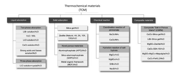
Figure 8. Thermochemical materials classification. Adapted from Yu et al. [47].
