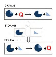
Figure 6. Scheme of thermochemical energy storage.
