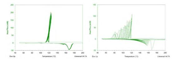
Figure 13. DSC response comparison between totally filled D-mannitol crucible (left) and partially filled D-mannitol crucible (right)<sup>1</sup>.
