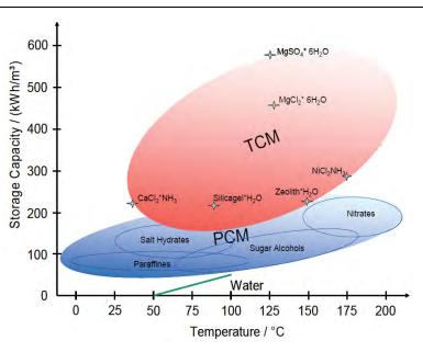
Figure 1. Storage capacity vs. Temperature for sensible (water), latent (PCM), and thermochemical (TCM) TES [2].
