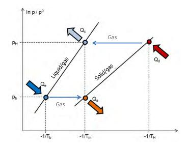
Figure 9. Diagram of Clausius–Clapeyron showing operation principle of a gas-solid TCM in a closed reactor [45].
