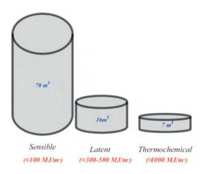
Figure 2. Volume needed to full cover the annual storage need of an energy efficient passive house (6480 MJ) [6].
