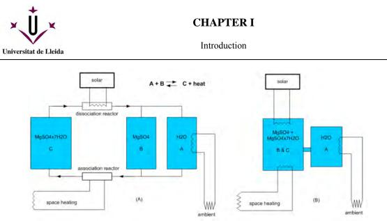
Figure 11. (a) separated reactor, (b) reactor integrated in storage [57].
