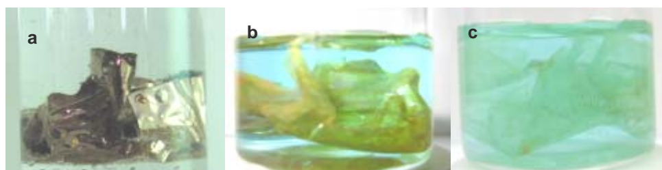
Fig 1. Light photographs of gradual changes of SPEEK membranes during different periods of time ( t_i ) in course of second loading with \text{Cu}^{2+} ions: a) t=0 , b) t=t_1 and c) t=t_2 . t_2 > t_1
