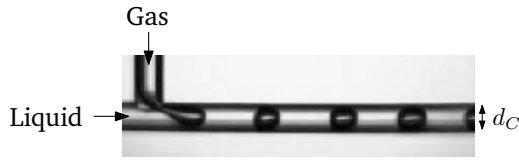
Figure 2.2: Illustration of the bubble generation method.
