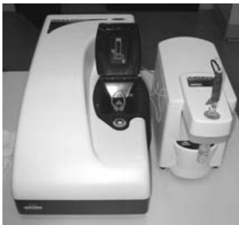
Figure 7.3. Photograph of the Zetasizer Nano ZS instrument (Malvern) (left) and the MPT-2 Autotitrator (right).
