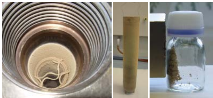
Figure 4.11. Photographs of SiFe_hexane products before being collected from the autoclave (left image), onto the Pyrex walls (middle image) and being attracted by a 0.5 Tesla magnet (right image).
