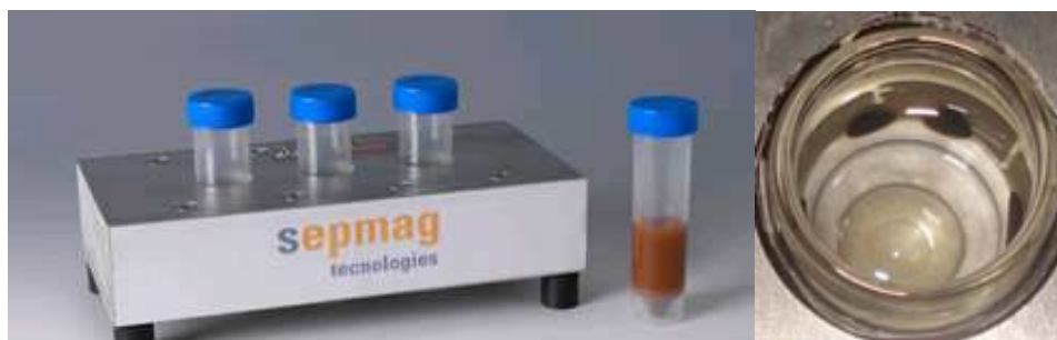
Figure 1.17. Lab-scale Precision Magnetophoresis system by Sepmag (left image) and one of our samples magnetically separated by the previous instrument (right image). 104
