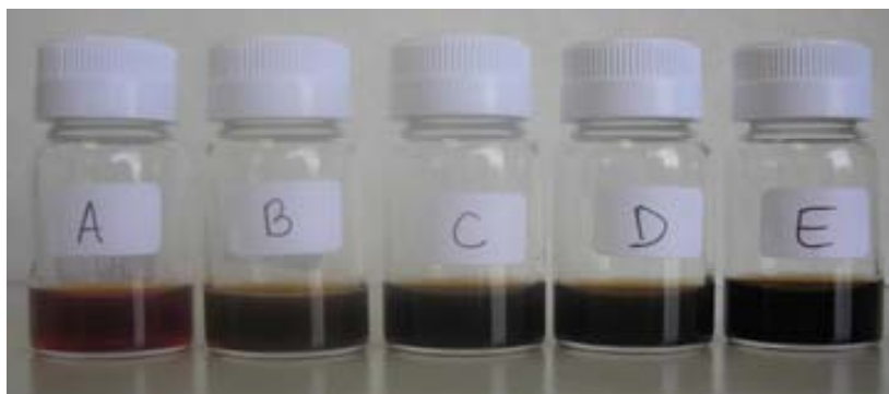
Figure 2.3. Photographs of several iron oxide colloidal dispersions.
