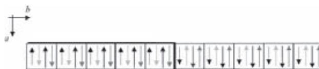
Figure 9. Simplified schematic representation of the square-wave magnetic structure of the LT phase of \epsilon -Fe 2 O 3 . The magnetic moments of the Fe DO1 , Fe DO2 , Fe RO , and Fe T sites are schematically represented by black, gray, light gray, and dotted arrows, respectively.
