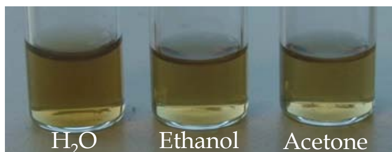
Figure 4.21. Photograph of sample SiFe_08_3 stabilized in several solvents at 1 mg composite/ml.
