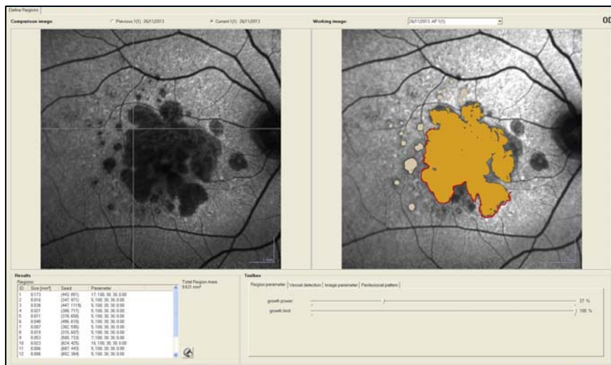
Figure 5. Region Finder ® screenshot. The user clicks on the hypoautofluorescent locations and the software automatically identifies regions with similar grey-scale levels (orange color on right-hand image), and converts the number of pixels identified into mm 2 . In case of software error, the user can define the borders of atrophy manually (red line on right-hand image).
