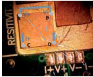
Figure A.8: Example of four point method for the measurement of sample resistivity
