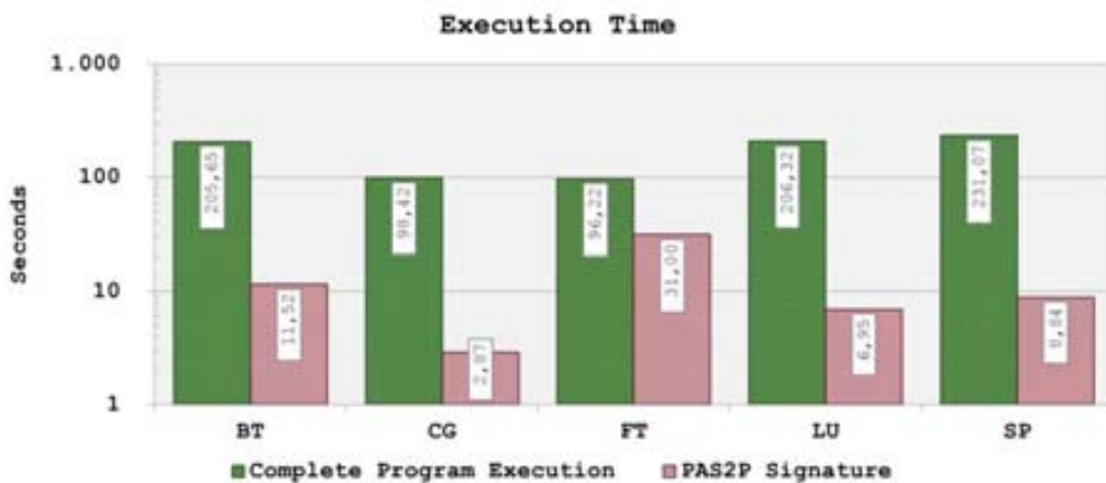
Figure 45 – Execution time comparison between complete program and PAS2P signature.
