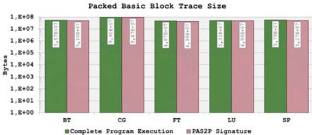
Figure 49 – Packed basic block trace size for complete program and PAS2P signature.
