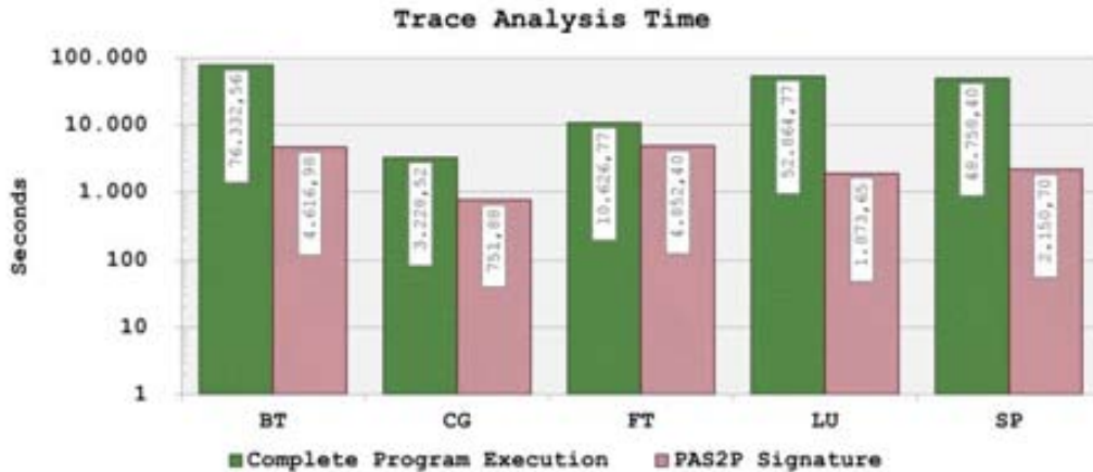
Figure 50 – Trace analysis time for complete program and PAS2P signature.
