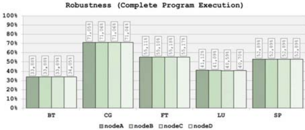
Figure 53 – Per process robustness for complete program execution.
