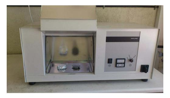
**Figure II-7** Atlas SUNTEST® instrument used to simulate solar irradiation and the Petri plates with *Prestige* oil (dark control is wrapped in Al foil).
