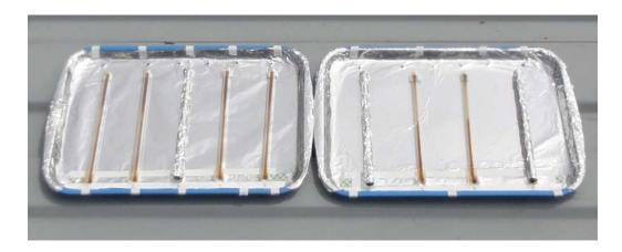
Figure II-8 Quartz tubes containing *MW* oil were exposed to natural sunlight.
