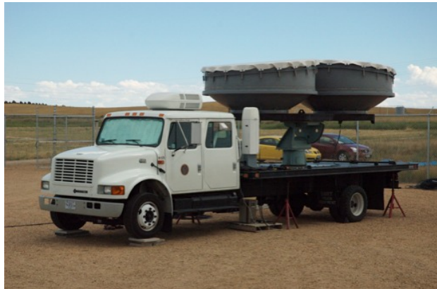
Figure 1.6: An S-band, FMCW atmospheric profiling radar from MIRSL. It employs separate antennas for transmitting and receiving. A Vaisala CL-31 lidar ceilometer is also contained within the white housing next to the antennas. Source: MIRSL [2014].
