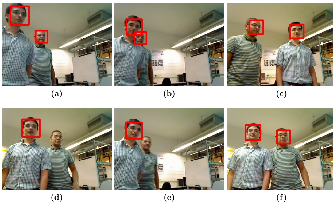
Figure 2.4: Results with 320x240 real-time images with Logitech QuickCam Orbit/Sphere AF. (a-c) Detected faces based on HF features. (e-f) Detected faces based on LBP features.
