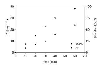
Figure 7.14: Evolution of chlorine ion and DCP removal as function of reaction time  $[H_2O_2]_i=85 \text{ mg.L}^{-1}$ ,  $[Fe(II)]_i=10 \text{ mg.L}^{-1}$  and free pH evolution.
