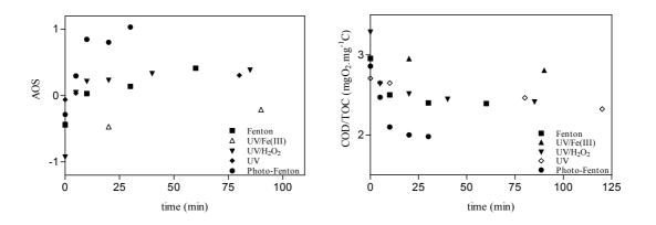
Figure 7.77: Change in oxidation state for the five processes during DCP photo-degradation.  $[H_2O_2]_i = 50$  mg.L<sup>-1</sup>,  $[Fe(II)]_i = 10$  mg.L<sup>-1</sup>,  $[Fe(III)]_i = 70$  mg.L<sup>-1</sup> and free pH evolution.
