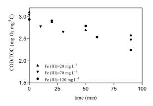
Figure 8.15: Evolution of COD/TOC as function of reaction time in UVA/Fe(III) process, for different initial Fe(III) concentrations in single lamp reactor.
