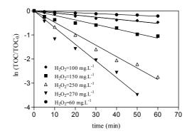
Figure 7.62: First order mineralization kinetics for DCP degradation.  $[Fe(II)]_i = 40 \text{ mg.L}^{-1}$ , and free pH evolution.
