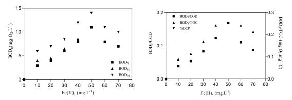
Figure 7.41: BOD<sub>n</sub>, BOD<sub>5</sub>/COD and BOD<sub>5</sub>/TOC as function of initial Fe (II) concentration for DCP in photo-Fenton,  $[H_2O_2]_i=30 \text{ mg-L}^{-1}$ , 40 min reaction time.
