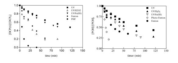
(A) (B) Figure 7.74. Comparison of the different processes for DCP and POH removal. A) DCP,  $[H_2O_2]_i = 50$ mg.L<sup>-1</sup>,  $[Fe(II)]_i = 10$  mg.L<sup>-1</sup>,  $[Fe(III)]_i = 70$  mg.L<sup>-1</sup> and free pH evolution, B) POH,  $[H_2O_2]_i = 30$  mg.L<sup>-1</sup>,  $[Fe(II)]_i = 10$  mg.L<sup>-1</sup>,  $[Fe(III)]_i = 70$  mg.L<sup>-1</sup> and free pH evolution
