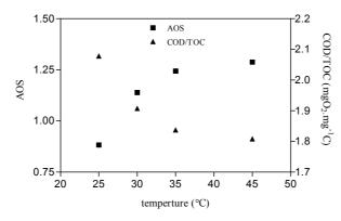
Figure 8.48: AOS and COD/TOC as function of operational temperature in photo-Fenton reaction.  $[H_2O_2]_i = 30 \text{ mg.L}^{-1}$ ,  $[Fe(II)]_i = 10$ , 50 min irradiation time and free pH evolution.
