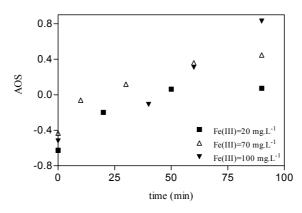
Figure 8.16: Evolution of AOS as function of reaction time in UVA/Fe(III) process, for different initial Fe(III) concentrations in multi lamps reactor.
