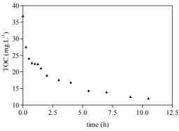
Figure 9.6: TOC evolution in aerobic SBR reactor during cycle of 12 h and feed BOD<sub>5</sub>/COD= 0.25
