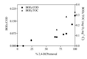
Figure 7.40: BOD<sub>5</sub>/COD and BOD<sub>5</sub>/TOC as a function DCP removal percentage.  $[H_2 O_2]_i = 50 \text{ mg.L}^{-1}$ ,  $[Fe(II)]_i = 10 \text{ mg.L}^{-1} 40 \text{ min and free pH evolution.}$
