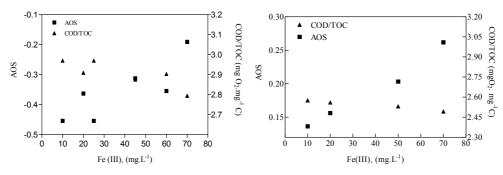
Figure 7.11: Evolution of COD/TOC and AOS as a function of initial Fe (III) concentration for DCP and POH in UV/Fe (III) process. Reaction time 90 min.
