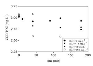
Figure 8.8: Evolution of COD/TOC vs. reaction time for  $UV/H_2O_2$  process at different initial  $H_2O_2$  concentrations in single lamp reactor.
