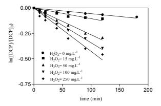
Figure 8.5: First order kinetics for DCP degradation by UVA/ $H_2$  O<sub>2</sub> process. At different  $H_2O_2$  initial concentration in single lamp reactor
