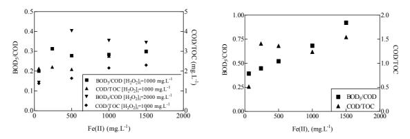
Figure 7.53: Evolution of the biodegradability and state of oxidation Vs. Fe(II) concentration at A)  $[H_2O_2]=1000$  and 2000 mg.L<sup>-1</sup>, B)  $[H_2O_2]=1000$  mg.L<sup>-1</sup> for photo-Fenton effluent solution,  $[POH]_i=1000$  mg.L<sup>-1</sup>, 15 min irradiation time and free pH evolutions.
