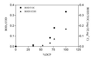
Figure 7.44: BOD<sub>5</sub>/COD and BOD<sub>5</sub>/TOC change as a function DCP removal, [Fe (II)]  $_{i}$  = 30 mg. L<sup>-1</sup> and [H<sub>2</sub> O<sub>2</sub>]  $_{i}$  = 30 mg. L<sup>-1</sup> for 40 min and free pH evolution.
