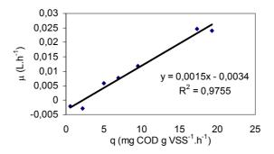
Figure 7.60: Evaluation of  $Y_{X/S}$  and  $k_d$  in the aerobic biological degradation for photo-Fenton pre-Treated solution. Initial conditions 100 mg.L<sup>-1</sup> POH, 50 mg.L<sup>-1</sup> H<sub>2</sub>O<sub>2</sub>, 75 mg.L<sup>-1</sup> Fe (II).
