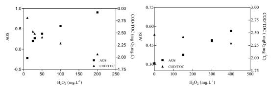
Figure 7.7: Evolution of COD/TOC and AOS as a function of initial  $H_2O_2$  concentration for DCP and POH in UV/  $H_2O_2$  process. Reaction time 90 min.
