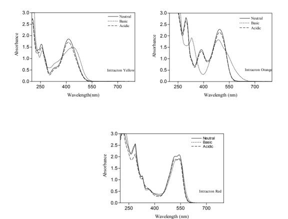
Figure 10.1: pH effect in UV-Vis. Spectra for intracron dyes
