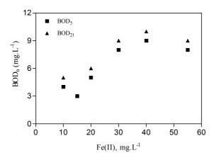
Figure 8.35 : BOD<sub>n</sub> as function of initial Fe(II) in single lamp photo-reactor.  $[H_2O_2]_i=30 \text{ mg.L}^{-1}$ , 50 min irradiation time and free pH evolution.
