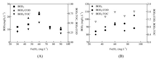
Figure 7.42: BOD<sub>5</sub>, BOD<sub>5</sub>/COD and BOD<sub>5</sub>/TOC as function of initial Fe (II) concentration for POH treated solution, A)  $[H_2O_2]_i = 50 \text{ mg-L}^{-1}$ , 15 min reaction time and free pH evolution, B)  $[H_2O_2]_i = 10 \text{ mg-L}^{-1}$ , 15 min reaction time and free pH evolution.
