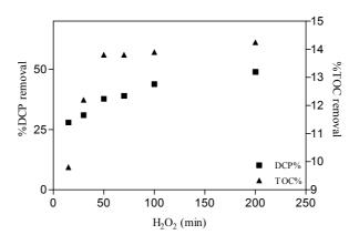
Figure 8.4: DCP and TOC removal percentage as function of  $H_2O_2$  in UVA/ $H_2O_2$  process for multi lamps reactor, irradiation time 2 hours.
