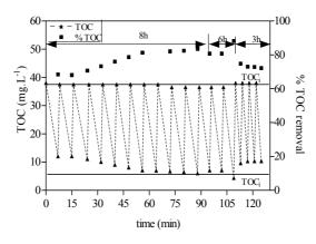
Figure 9.12: Evolution of initial organic carbon after feeding the reactor  $(TOC_i)$ , final organic carbon before next feeding  $(TOC_f)$  and organic mater removal for each cycle (%TOC) as function of time, cycle duration 8 h and feed BOD<sub>5</sub>/COD= 0.48.
