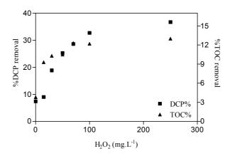
Figure 8.2: DCP and TOC removal percentage as function of  $H_2O_2$  in UVA/ $H_2O_2$  process for single lamp reactor, irradiation time 2 hours.
