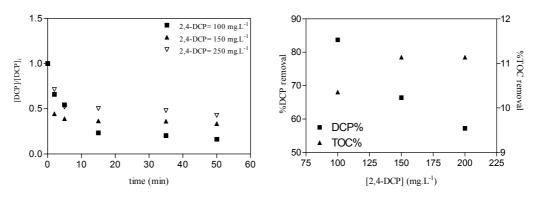
Figure 8.28: Evolution of DCP vs. irradiation time for different initial DCP for single lamp photo-reactor.  $[H_2O_2]_i = 30 \text{ mg.L}^{-1}$ ,  $[Fe(II)]_i = 10 \text{ mg.L}^{-1}$ .
