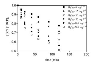
Figure 8.3: Evolution of DCP vs. reaction time for different  $H_2O_2$  initial concentration in UVA/ $H_2O_2$  process for multi lamps reactor.
