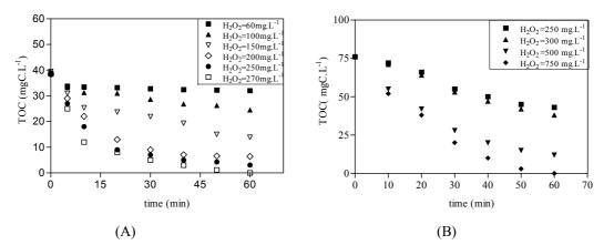
Figure 7.61: Mineralization of DCP and POH at different  $H_2O_2$  concentration, conditions A) [Fe (II)]<sub>i</sub>=40 mg.L<sup>-1</sup>, time=60 min and free pH evolution, B) [Fe (II)]<sub>i</sub>=60 mg.L<sup>-1</sup>, time=60 min and free pH evolution.
