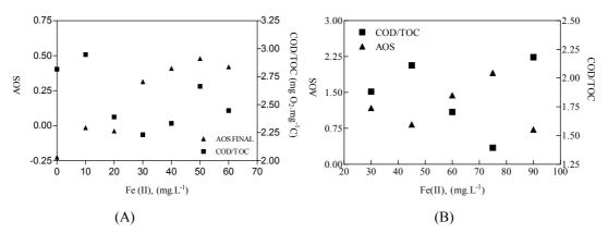
Figure 7.48: AOS and COD/TOC as function of initial Fe(II). Initial conditions, A) DCP  $[H_2O_2]_i = 10$  mg-L<sup>-1</sup>, 40 min reaction time and B) POH  $[H_2O_2]_i = 50$  mg-L<sup>-1</sup>, 15 min reaction time.
