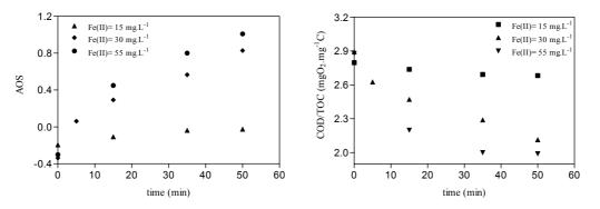
Figure 8.44: AOS and COD/TOC as function of time at different initial Fe(II) in single lamp photo-reactor.[H<sub>2</sub>O<sub>2</sub>] = 30 mg.L<sup>-1</sup>, 50 min irradiation time and free pH evolution.
