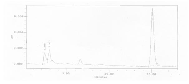
Figure A5.2: Chromatogram corresponding to sample at 30 min in UVA/H<sub>2</sub>O<sub>2</sub> process
