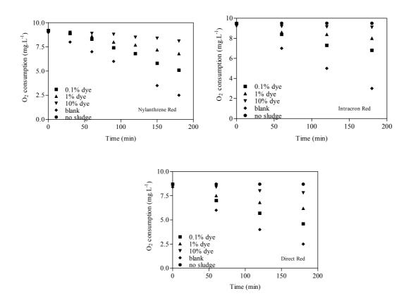
Figure 10.4 : Inhibition of  $O_2$  consumption by activated sludge for three dye solutions (100mg.L  $^{-1},\,pH=$  7.0± 0.2 )
