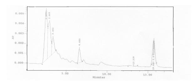
Figure A5.4: Chromatogram corresponding to sample at 2 min in photo-Fenton process
