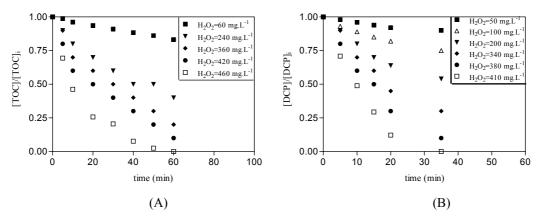
Figure 8.49: Normalized TOC evolution as function of time at different initial  $H_2O_2$  A) single lamp reactor B) multi lamps reactor.  $[Fe(II)]_i = 10 \text{ mg.L}^{-1}$  and Free pH evolution
