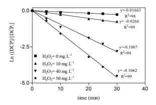
Figure 7.28: First-order plot for degradation of DCP as function of initial  $H_2 O_2$ . [Fe(II)]<sub>i</sub>=10 mg:L<sup>-1</sup> and free pH evolution.
