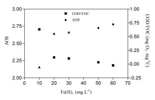
Figure 8.47: AOS and COD/TOC as function of initial Fe(II) in multi lamps photo-reactor.  $[H_2O_2]_i = 15$  mg.L<sup>-1</sup>, 50 min irradiation time and free pH evolution.
