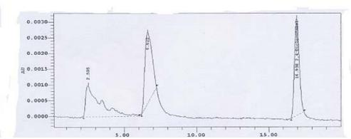
Figure 7.64: Chromatogram corresponding to sample at 90 min of direct UV-photolysis
