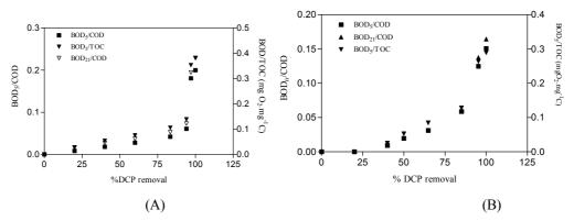
Figure 8.34: BOD<sub>5</sub>/COD and BOD<sub>5</sub>/TOC as a function DCP removal percentage A) single lamp reactor with  $[H_2 O_2]_i = 75 \text{ mg.L}^{-1}$ ,  $[Fe(II)]_i = 10 \text{ mg.L}^{-1} 50 \text{ min}$  and free pH evolution, B) multi lamps reactor with  $[H_2 O_2]_i = 65 \text{ mg.L}^{-1}$ ,  $[Fe(II)]_i = 10 \text{ mg.L}^{-1} 35 \text{ min}$  and free pH evolution.
