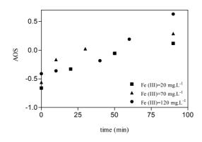
Figure 8.14: Evolution of AOS as function of reaction time in UVA/Fe(III) process, for different initial Fe(III) concentrations in single lamp reactor.
