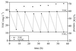
Figure 9.11: Evolution of initial organic carbon after feeding the reactor  $(TOC_i)$ , final organic carbon before next feeding  $(TOC_f)$  and organic mater removal for each cycle (%TOC) as function of time, cycle duration 8 h and feed BOD<sub>5</sub>/COD= 0.35.
