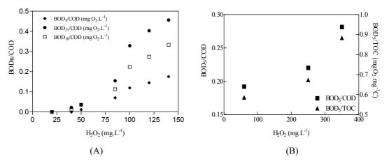
Figure 7.17: Change in Bon<sub>n</sub>/COD ratios as function of initial  $H_2O_2$  concentration in Fenton reaction. (A) DCP with  $[Fe(II)]_i = 10 \text{ mg.L}^{-1}$ , 60 min reaction time ((30 min for POH) and free pH evolution, (B)POH with  $Fe(II)]_i = 10 \text{ mg.L}^{-1}$ , 30 min reaction time and free pH evolution.
