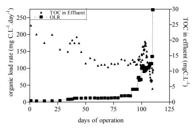
Figure 9.2: TOC in effluent solution as function of operation days for aerobic SBR. Feed BOD<sub>5</sub>/COD=0.25.
