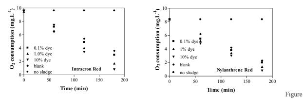
10.9: Inhibition of O<sub>2</sub> consumption by activated sludge for photolyzed Nylanthrene Red dye and Intracron Red dye (100mg.L<sup>-1</sup>, pH=7.0 $\pm$  0.2, irradiation time : 7.5 and 3.4 min respectively).
