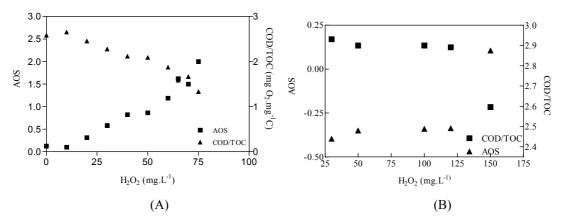
Figure 7.46: AOS and COD/TOC evolution as function of initial hydrogen peroxide (A) DCP. [Fe (II)]<sub>i</sub>= 10 mg.L<sup>-1</sup>, 40 min reaction time and free pH evolution .B) (A) POH , [Fe (II)]<sub>i</sub>= 10 mg.L<sup>-1</sup>, 15 min reaction time and free pH evolution .
