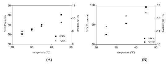
Figure 8.27: DCP% removal and TOC elimination for different initial temperature. A) single lamp reactor,  $[H_2O_2]_i = 30 \text{ mg.L}^{-1}, [Fe(II)]_i = 10 \text{ mg.L}^{-1}$ , free pH evolution and reaction time 50 B) multi lamps reactor,  $[H_2O_2]_i = 30 \text{ mg.L}^{-1}, [Fe(II)]_i = 10 \text{ mg.L}^{-1}$ , free pH evolution and reaction time 35 min
