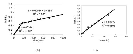
Figure 7.57: Kinetic study of the biodegradation of 100% pre-treated solution carried out in the acclimated reactor. Conditions: (A) T = 22°C, pH  $\approx$  7.2, TVSS = 0.13 g.L<sup>-1</sup>, HRT = 1 days, (B) (A) T = 22°C, pH  $\approx$  7.2, TVSS = 0.13 g.L<sup>-1</sup>, HRT = 12 h
