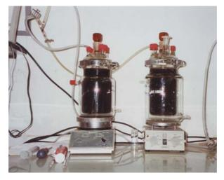
Figure 5.6 biological stirred tank reactors
