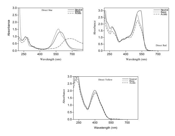
Figure 10.3: pH effect in UV-Vis. spectra for Optisal direct dyes
