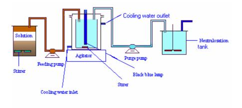
Figure 5.3; Single lamp stirred tank photo-reactors .
