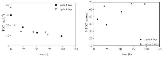
Figure 9.4: TOC evolution and organic matter removals (%TOC) as function of time for SBR operated at 4 and 3 days cycle duration , feed  $BOD_5/COD= 0.25$
