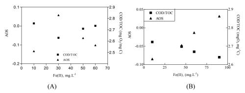
Figure 7.23: AOS and COD/TOC evolution of as a function of initial Fe (II) concentration for Fenton process. process (A) DCP  $[H_2O_2]_i = 20 \text{ mg.L}^{-1}$ , 60 min reaction time and free pH evolution, (B) POH  $[H_2O_2]_i = 30 \text{ mg.L}^{-1}$ , 30 min reaction time and free pH evolution,
