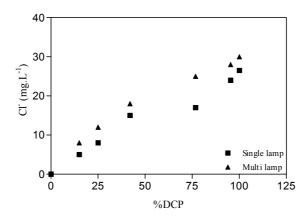
Figure 8.29: Dechlorination as function of DCP removal in single and multi lamps reactors.
