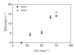
Figure 8.30: Evolution of  $BOD_n$  as function of initial  $H_2O_2$  in single lamp photo-reactor.[Fe(II)]<sub>i</sub>= 10 mg.L<sup>-1</sup>, 50 min irradiation time and free pH evolution.
