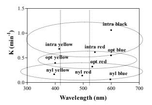
Figure 10.10 : Apparent kinetic constants vs.  $\lambda_{\text{max}}$  in the visible range.
