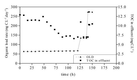
Figure 9.12 Evolution of total organic carbon (TOC) in effluent as function of operation hours.
