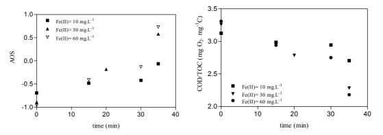
Figure 8.46: AOS and COD/TOC as function of time at different initial Fe(II) in multi lamps photo-reactor.[H<sub>2</sub>O<sub>2</sub>] = 15 mg.L<sup>-1</sup>, 50 min irradiation time and free pH evolution.
