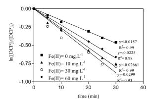
Figure 7.31: First-order plot for degradation of DCP as function of initial Fe (II) in photo-Fenton reaction: $[H_2O_2]_I = 10 \text{ mg.L}^{-1}$  and free pH evolutions.
