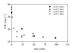
Figure 9.17: Evolution of organic matter as function of cycle duration, cycle duration 4,3, 2 and 1 day and feed  $BOD_5/COD = 0.25$ .
