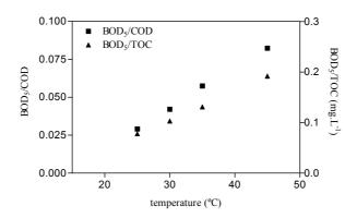
Figure 8.39: Variation of biodegradability as function of operational temperature in single lamp photo-reactor.  $[H_2O_2]_i= 30 \text{ mg.L}^{-1}, [Fe(II)]_i= 10 \text{ mg.L}^{-1}, 50 \text{ min irradiation time and free pH evolution.}$
