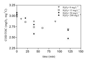
Figure 8.10: Evolution of COD/TOC vs. reaction time for  $UVA/H_2O_2$  process at different initial  $H_2O_2$  concentrations in multi lamps reactor.
