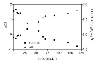
Figure 8.43: AOS and COD/TOC as function of initial  $H_2O_2$  in single lamp photo- reactor.  $[Fe(II)]_i = 10$  mg.L<sup>-1</sup>, 35 min irradiation time and free pH evolution.
