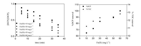
Figure 8.26: DCP degradation as function of iron catalyst in photo-Fenton process in multi lamps reactor.  $[H_2O_2]_i=15 \text{ mg.L}^{-1}$  and 35 min irradiation.
