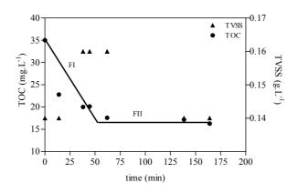
Figure 9.3: Evolution of TOC and TVSS as function of cycle duration, cycle duration 8 days and feed  $BOD_5/COD= 0.21$ .
