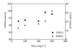
Figure 7.26: POH degradation in photo-Fenton reaction and different initial  $H_2O_2$  concentrations. [Fe (II)]<sub>i</sub>=60 mg. L<sup>-1</sup>,free pH evolution, 15 min reaction time.
