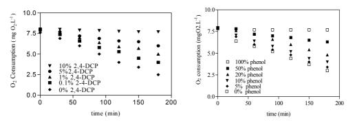
Figure 7.3: Inhibition test of oxygen consumption by activated sludge for 100 mg.L<sup>-1</sup> DCP and 100 mg.L<sup>-1</sup> POH solution.
