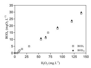
Figure 8.31: Evolution of BOD<sub>n</sub> as function of initial  $H_2O_2$  in multi lamps photo-reactor.[Fe(II)]<sub>i</sub>= 10 mg.L<sup>-1</sup>, 35 min irradiation time and free pH evolution.
