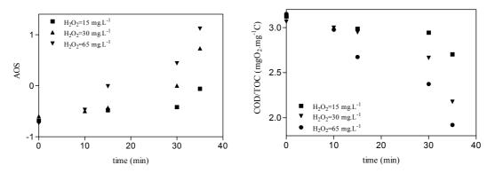
Figure 8.42: AOS and COD/TOC as function of time for different initial  $H_2O_2$  in multi lamps photo-reactor.[Fe(II)]<sub>i</sub>= 10 mg.L<sup>-1</sup>, 35 min irradiation time and free pH evolution.
