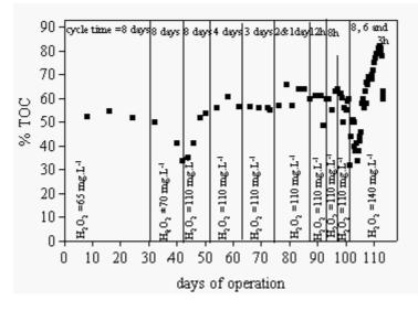
Figure 9.14: TOC removal as function of time at different initial H<sub>2</sub>O<sub>2</sub> used in photo-Fenton and cycle duration.
