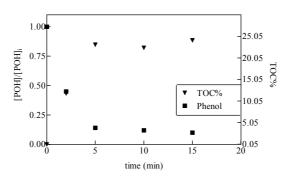
Figure 7.51: Variation of POH concentration and TOC removal percentage COD/TOC and ratio for photo-Fenton effluent solution (1000 mg.L<sup>-1</sup> POH, 3000 mg.L<sup>-1</sup> H<sub>2</sub>O<sub>2</sub> and 1500 mg.L<sup>-1</sup> Fe(II))
