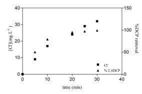
Figure 7.36: Evolution of chloride ion and DCP % elimination as function of reaction time.  $[H_2O_2]=50$  mg.L<sup>-1</sup>, [Fe(II)]=10 mg.L<sup>-1</sup>.
