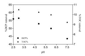
Figure 7.32: Evolution of DCP degradation as function of pH,  $[H_2O_2]_i = 10 \text{ mg.L}^{-1}$ ,  $[Fe (II)]_i = 10 \text{ mg.L}^{-1}$  and reaction time 40 min.
