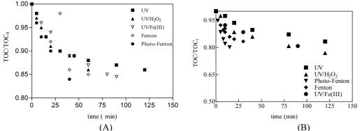
Figure 7.75: TOC mineralization for different AOP's. A) DCP,  $[H_2O_2]_i = 50 \text{ mg.L}^{-1}$ ,  $[Fe(II)]_i = 10 \text{ mg.L}^{-1}$ ,  $[Fe(III)]_i = 70 \text{ mg.L}^{-1}$  and free pH evolution, B) POH,  $[H_2O_2]_i = 30 \text{ mg.L}^{-1}$ ,  $[Fe(II)]_i = 10 \text{ mg.L}^{-1}$ ,  $[Fe(III)]_i = 70 \text{ mg.L}^{-1}$  and free pH evolution
