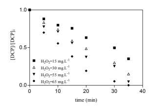
Figure 8.20. Evolution of DCP as function of irradiation time at different  $H_2O_2$  in multi lamps photoreactor.  $[Fe(II)]_i = 10 \text{ mg. L}^{-1}$
