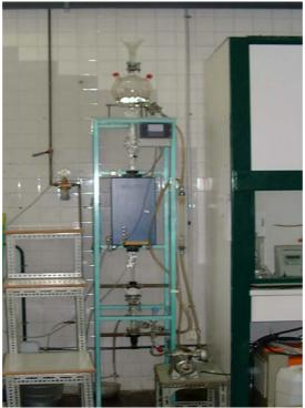
Figure (5.1b) Tubular photo- reactor
