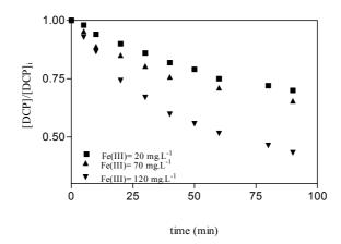
Figure 8.11 Evolution of DCP vs. reaction time at different initial Fe(III) concentrations in UVA/Fe(III) process in single lamp reactor.
