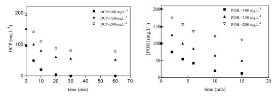
Figure 7.33: DCP and POH evolution as function of time for different initial concentrations, initial condition; for DCP are  $[H_2O_2]_i = 50 \text{ mg.L}^{-1} [Fe(II)]_i = 10 \text{ mg.L}^{-1}$  and free pH evolution, for POH  $[H_2O_2]_i = 50 \text{ mg.L}^{-1} [Fe(II)]_i = 60 \text{ mg.L}^{-1}$ .
