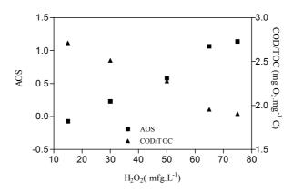
Figure 8.41: AOS and COD/TOC as function of initial  $H_2O_2$  in single lamp photo- reactor.  $[Fe(II)]_i = 10$  mg.L<sup>1</sup>, 50 min irradiation time and free pH evolution.
