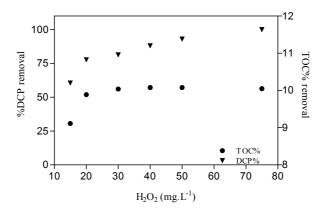
Figure 8.19: DCP removal as function of different initial  $H_2O_2$  concentration in single lamp photoreactor  $[Fe(II)]_i = 10 \text{ mg. } L^{-1} \text{ or}$
