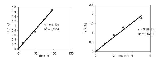
Figure 7.59: Kinetic study of aerobic biodegradation of A) POH, B) photo-Fenton effluent solution 100 mg.L<sup>-1</sup> POH, 50 mg.L<sup>-1</sup> H<sub>2</sub>O<sub>2</sub>, 75 mg.L<sup>-1</sup> Fe<sup>+2</sup>
