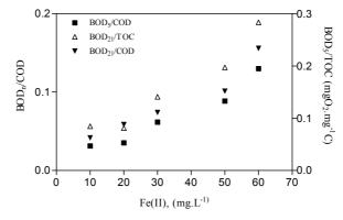
Figure 8.38:  $BOD_n/COD$  and  $BOD_5/TOC$  as function of initial Fe(II) in multi lamp photo-reactor.  $[H_2O_2]_i = 15 \text{ mg.L}^{-1}$ , 35 min irradiation time and free pH evolution.
