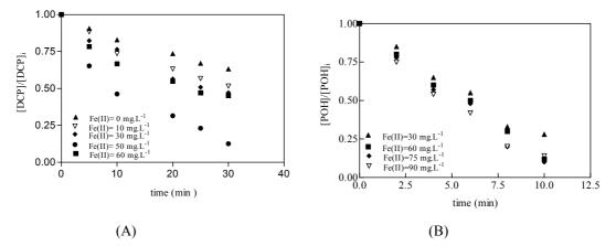
Figure 7.29: DCP and POH degradation as function of time for different Fe (II) initial concentration. (A)  $[H_2O_2]_i = 10 \text{ mg.L}^{-1}$  and experimental time 40 min. (B)  $[H_2O_2]_i = 50 \text{ mg.L}^{-1}$  and experimental time 15min and free pH evolution.
