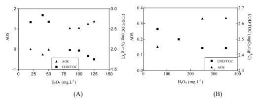
Figure 7.22: AOS and COD/TOC evolution of as a function of initial  $H_2O_2$  concentration for modified Fenton process (A) DCP [Fe (II)]<sub>i</sub> = 10 mg.L<sup>-1</sup>, 60 min reaction time and free pH evolution, (B) POH [Fe (II)]<sub>i</sub> = 10, 30 min reaction time and free pH evolution
