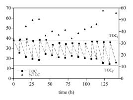
Figure 9.18: Evolution of initial organic carbon after feeding the reactor  $(TOC_i)$ , final organic carbon before next feeding  $(TOC_f)$  and organic mater removal for each cycle (%TOC) as function of time, cycle duration 8h and feed  $BOD_5/COD= 0.25$ .
