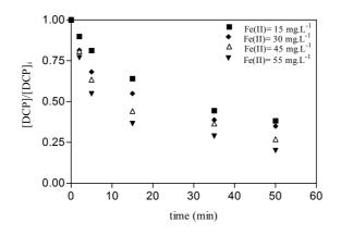
Figure 8.22: Evolution of normalized DCP concentration as function of time at different initial Fe(II) concentration in single lamp reactor.  $[H_2O_2]_i = 15 \text{ mg.L}^{-1}$
