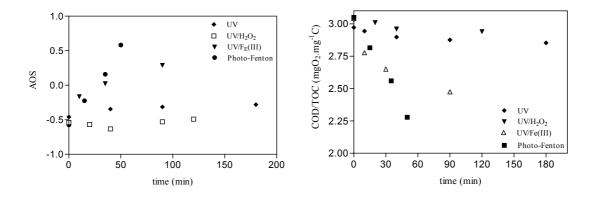
Figure 8.54: Change in oxidation state for the five AOP's, in single lamp photo-reactor.  $[H_2O_2]_i = 50$  mg.L<sup>-1</sup>,  $[Fe(III)]_i = 70$  mg.L<sup>-1</sup>,  $.[Fe(II)]_i = 10$  mg.L<sup>-1</sup>, and free pH evolutions.
