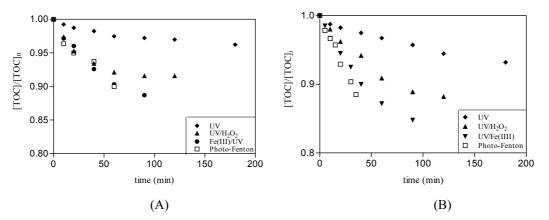
Figure 8.52: Normalized TOC concentrations as function of time for the different AOP's processes, A) single lamp, B) multi lamps reactor.  $[H_2O_2]_i = 50 \text{ mg.L}^{-1}$ ,  $[Fe(III)]_i = 70 \text{ mg.L}^{-1}$ ,  $[Fe(II)]_i = 10 \text{ mg.L}^{-1}$  and free pH evolution.
