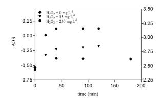
Figure 8.7 Evolution of AOS vs. reaction time for UVA/H<sub>2</sub>O<sub>2</sub> process at different initial H<sub>2</sub>O<sub>2</sub> concentrations in single lamp reactor.
