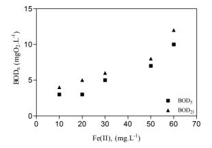
Figure 8.36 : BOD<sub>n</sub> as function of initial Fe(II) in multi lamps photo-reactor.  $[H_2O_2]_i$ = 15 mg.L<sup>-1</sup>, 35 min irradiation time and free pH evolution.
