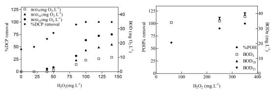
Figure 7.15: Evolution of  $BOD_n$ , DCP removal and POH removal as function of initial  $H_2O_2$  in Fenton reaction.  $[Fe(II)]_i = 10, 60$  min reaction time (30 min for POH) and free pH evolution.
