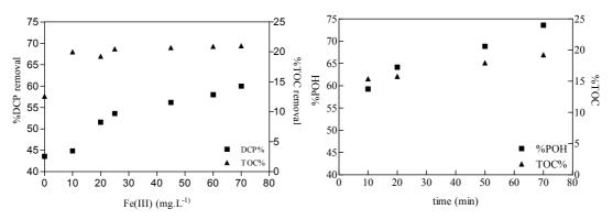
Figure 7.8: Evolution of DCP, POH and TOC as function of initial Fe (III) concentration during UV/ Fe (III) process. Reaction time 90 min
