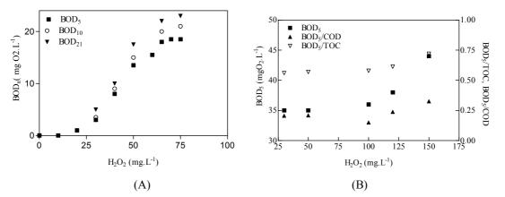
Figure 7.37: BOD<sub>n</sub> as function of initial  $H_2O_2$  concentration for A) DCP Initial conditions, DCP are [Fe (II)]<sub>i</sub>= 10 mg-L<sup>-1</sup>, 40 min reaction time and POH solution treated by photo-Fenton. and B)POH Initial conditions, [Fe(II)]<sub>i</sub>= 10 mg-L<sup>-1</sup>, 15 min.
