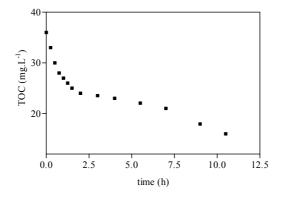
Figure 9.18: Evolution of organic matter as function of cycle duration (12h), and feed BOD<sub>5</sub>/COD =0.25.
