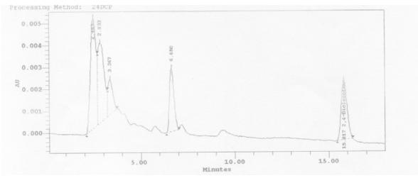
Figure A5.5: Chromatogram corresponding to sample at 20 min in photo-Fenton process
