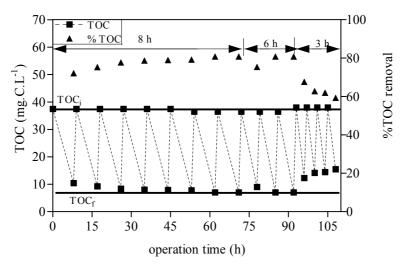
Figure 9.19: Evolution of initial organic carbon after feeding the reactor (TOC<sub>i</sub>), final organic carbon before next feeding (TOC<sub>f</sub>) and organic mater removal for each cycle (%TOC) as function of time, cycle duration 8. 6 and 3 h and feed BOD<sub>5</sub>/COD= 0.48.
