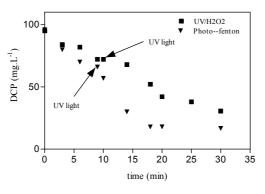
Figure 7.35:Variation of DCP as function of UV irradiation time for:  $UV/H_2 O_2$  and photo-Fenton processes,  $[H_2 O_2]_i=30 \text{ mg.L}^{-1}$ ,  $[Fe (II)]_i=10 \text{ mg.L}^{-1}$
