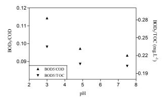
Figure 7.45: Change of BOD<sub>5</sub>/COD and BOD<sub>5</sub>/TOC as function of initial pH. [Fe (II)]<sub>i</sub>=10 mg.L<sup>-1</sup> and [H<sub>2</sub>  $O_2$ ]<sub>i</sub>= 30 mg.L<sup>-1</sup> and 40min experimental time
