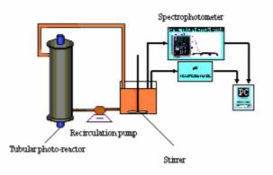
Figure 5.5: Tubular photo-reactor.
