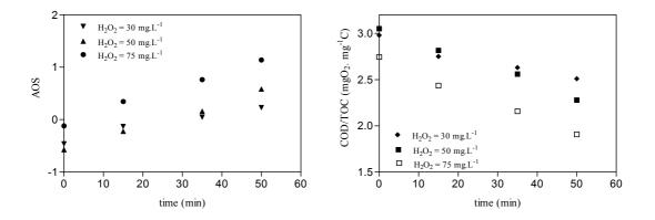
Figure 8.40: AOS and COD/TOC as function of time for different initial  $H_2O_2$  in single lamp photo-reactor.[Fe(II)]<sub>i</sub>= 10 mg.L<sup>-1</sup>, 50 min irradiation time and free pH evolution.
