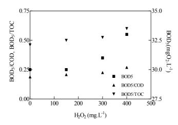
Figure 7.6: BOD<sub>5</sub>, BOD<sub>5</sub>/TOC and BOD<sub>5</sub>/COD Evolution of POH treated solution with UV/H<sub>2</sub>O<sub>2</sub> process
