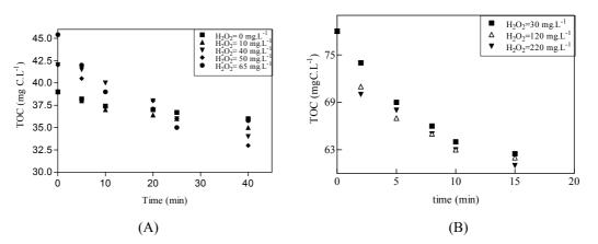
Figure 7.25: Total organic carbon evolution (TOC) in photo-Fenton reaction and different initial  $H_2O_2$  concentrations, A) DCP and B) POH. [Fe (II)]<sub>i</sub>=10 mg. L<sup>-1</sup>, free pH evolution.
