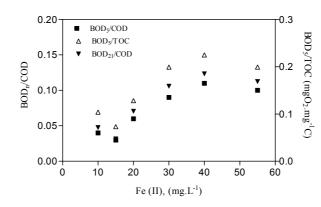
Figure 8.37 : BOD<sub>n</sub>/COD and BOD<sub>5</sub>/TOC as function of initial Fe(II) in single lamp photo-reactor.  $[H_2O_2]_i=30 \text{ mg.L}^{-1}$ , 50 min irradiation time and free pH evolution.
