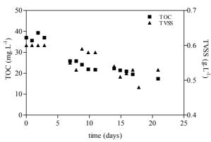
Figure 9.15: Total organic carbon (TOC) evolution and biomass concentration (TVSS) as function of acclimation time, feed  $BOD_5/COD = 0.15$ .
