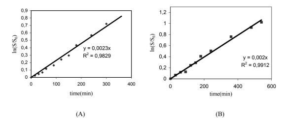
Figure 7.55. Kinetic study of the biodegradation of 100% pre-treated solution carried out in the non-acclimated reactor. Conditions:  $T = 22^{\circ}C$ , pH  $\approx$  7.2, TVSS = 0.35 g.L<sup>-1</sup>, (A)HRT = 2 days and (B) T = 22°C, pH  $\approx$  7.2, TVSS = 0.35 g.L<sup>-</sup> HRT = 1 days.
