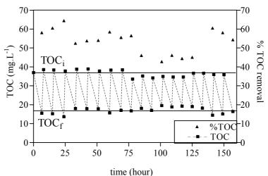
Figure 9.7: Evolution of initial organic carbon after recording the reactor (TOC<sub>i</sub>), final organic carbon before next feeding (TOC<sub>f</sub>) and organic mater removal for each cycle (%TOC) as function of time, cycle duration 8 h and feed BOD<sub>5</sub>/COD= 0.25.
