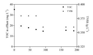
Figure 9.16: Evolution of organic matter and biomass concentration as function of cycle duration, cycle duration 8 days and feed  $BOD_5/COD = 0.15$ .
