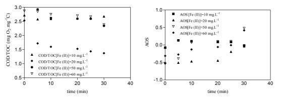
Figure 7.50: AOS and COD/TOC Evolution as reaction time for different initial Fe (II). Concentrations.  $[H_2O_2]_i = 10 \text{ mg.L}^{-1}$  and free pH evolutions
