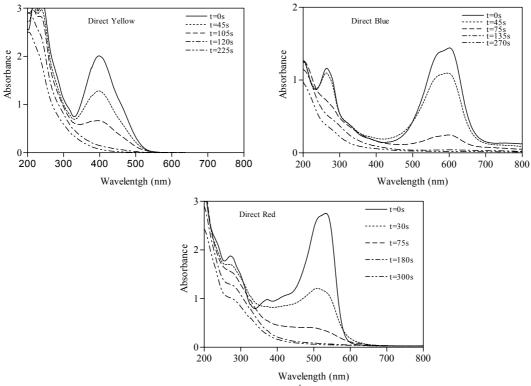
Figure 10.5 : UV photolysis of Optisal dyes (100 mg.L<sup>-1</sup>).
