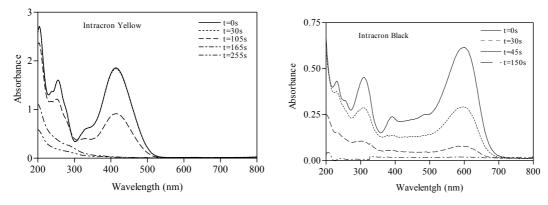
Figure 10.6 : UV Photolysis of Intracron reactive dyes (100 mg.L<sup>-1</sup>).
