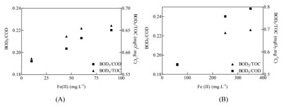
Figure 7.20: Change in BOD<sub>5</sub>/TOC and BOD<sub>5</sub>/COD ratios as function of initial Fe (II) concentration for POH treated in A)Fenton and B) modified Fenton reactions.  $[H_2O_2]_i = 20 \text{ mg.L}^{-1}$ , 30 min reaction time and free pH evolution
