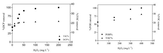
Figure 7.4: DCP, POH and TOC removal as function of initial  $H_2O_2$  concentration during UV/  $H_2O_2$  process. Reaction time 90 min .
