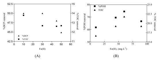
Figure 7.13: Evolution of DCP, POH and TOC removals as function of initial Fe (II) in Fenton process. (A)  $[H_2O_2]_i = 20 \text{ mg.L}^{-1}$ , 60 min reaction time and free pH evolution, (B) (A)  $[H_2O_2]_i = 30 \text{ mg.L}^{-1}$ , 30 min reaction time and free pH evolution.
