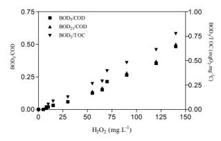
Figure 8.33: Evolution of  $BOD_n/COD$  and  $BOD_n/TOC$  as function of initial  $H_2O_2$  in multi lamps photoreactor.[Fe(II)]<sub>i</sub>= 10 mg.L<sup>-1</sup>, 35 min irradiation time and free pH evolution
