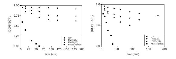
Figure 8.50: DCP evolution as function of time for different AOP's in single and multi lamps reactor.  $[H_2O_2]_i = 50 \text{ mg.L}^{-1}$ ,  $[Fe(III)]_i = 70 \text{ mg.L}^{-1}$ ,  $[Fe(III)]_i = 10 \text{ mg.L}^{-1}$  and free ph evolution.
