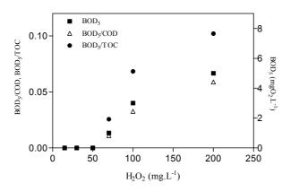
Figure 8.6: BOD<sub>5</sub>, BOD<sub>5</sub>/COD and BOD<sub>5</sub>/TOC as function of initial  $H_2O_2$  in UVA/ $H_2O_2$  for multi lamps reactor, reaction time 90 min.
