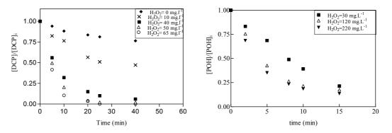
Figure 7.24: DCP and POH degradation in photo-Fenton reaction at different initial  $H_2O_2$  concentrations. [Fe (II)]<sub>i</sub>=10 mg. L<sup>-1</sup>, free pH evolution.
