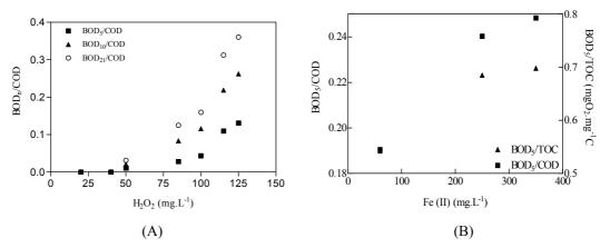
Figure 7.18: Change in  $BOD_n/COD$  ratios as function of initial  $H_2O_2$  concentration for modified Fenton reaction. (A) DCP with  $[Fe(II)]_i = 10 \text{ mg.L}^{-1}$ , 60 min reaction time ((30 min for POH) and free pH evolution, (B)POH with  $Fe(II)]_i = 10 \text{ mg.L}^{-1}$ , 30 min reaction time and free pH evolution.
