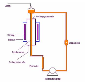
Figure (5.1 a) Tubular Photo- reactor
