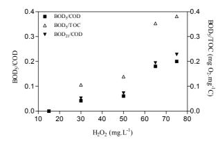
Figure 8.32: Evolution of  $BOD_n/COD$  and  $BOD_n/TOC$  as function of initial  $H_2O_2$  in single lamp photo-reactor.[Fe(II)]<sub>i</sub>= 10 mg.L<sup>-1</sup>, 50 min irradiation time and free pH evolution.
