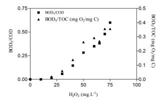
Figure 7.38: BOD<sub>5</sub>/COD and BOD<sub>5</sub>/TOC as function of initial  $H_2O_2$  concentration for DCP solution. [Fe (II)]<sub>i</sub>= 10 mg-L<sup>-1</sup>, 40 min reaction time.
