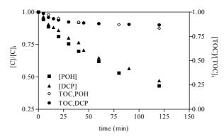
Figure 7.1: Normalized concentrations of DCP, POH and change in TOC Vs. irradiation time in direct UV-light photolysis.
