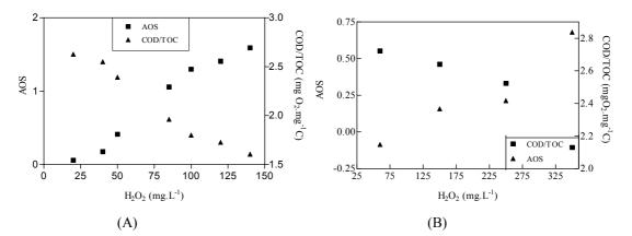
Figure 7.21: AOS and COD/TOC evolution of as a function of initial  $H_2O_2$  concentration for Fenton process. process (A) DCP [Fe (II)]<sub>i</sub> = 10 mg.L<sup>-1</sup>, 60 min reaction time and free pH evolution, (B) POH [Fe (II)]<sub>i</sub> = 10, 30 min reaction time and free pH evolution
