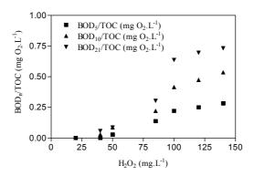
Figure 7.19: Change in  $BOD_n/TOC$  ratios as function of initial  $H_2O_2$  concentration for DCP in Fenton and modified Fenton reactions. [Fe (II)]<sub>i</sub> or [Fe (III)]<sub>i</sub> = 10 mg.L<sup>-1</sup>, 60 min reaction time and free pH evolution.
