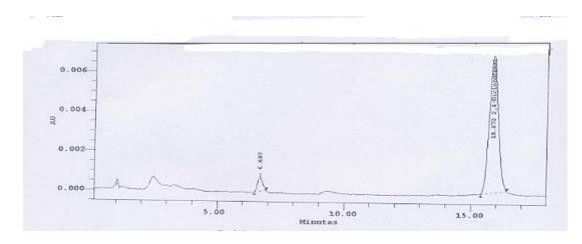
Figure 7.70: Chromatogram corresponding to sample at 0.5 min of photo-Fenton reaction
