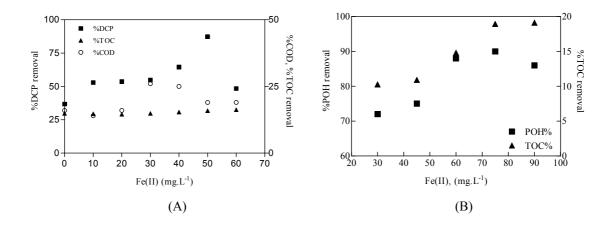
Figure 7.30: DCP, POH and TOC removal percentages as function of initial Fe(II). (A)  $[H_2O_2]_i = 10$  mg.L<sup>-1</sup> and reaction time 40 min. (B)  $[H_2O_2]_i = 50$  mg.L<sup>-1</sup> and reaction time 15min and free pH evolution.
