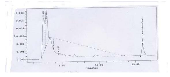
Figure 7.66 Chromatogram corresponding to sample at 30 min of direct UV/H<sub>2</sub>O<sub>2</sub> photolysis
