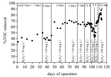
Figure 9.14: TOC removal as function of time at different initial  $H_2O_2$  used in photo-Fenton and cycle duration.
