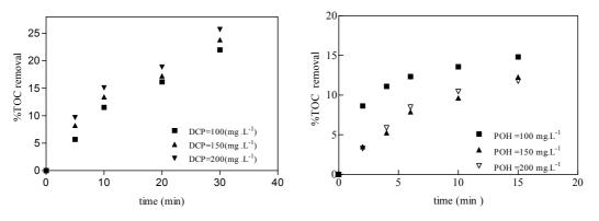
Figure 7.34: Evolution of TOC vs. reaction time for different DCP and POH initial concentrations, initial condition; for DCP are  $[H_2O_2]_i = 50 \text{ mg.L}^{-1} [Fe(II)]_i = 10 \text{ mg.L}^{-1}$  and free pH evolution, for POH  $[H_2O_2]_i = 50 \text{ mg.L}^{-1} [Fe(II)]_i = 60 \text{ mg.L}^{-1}$ .
