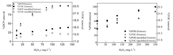
Figure 7.12: Evolution of DCP, POH and TOC removal in Fenton and modified Fenton as function of initial  $H_2O_2$  [Fe (II)]<sub>i</sub> or [Fe (III)]<sub>i</sub> =10 mg.L<sup>-1</sup> and 60 min reaction time (30 min in POH case)
