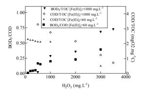
Figure 7.52: Evolution of the biodegradability and oxidation state Vs.  $H_2O_2$  concentration at Fe(II)=60 mg.L<sup>-1</sup> for photo-Fenton effluent solution, [POH]<sub>i</sub>=1000 mg.L<sup>-1</sup>, pH<sub>0</sub>=3
