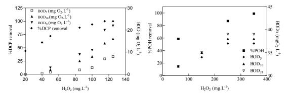
Figure 7.16:  $BOD_n$ , DCP removal and POH removal removals percentage evolution as function of initial  $H_2O_2$  in modified Fenton reaction. [Fe (III)]<sub>i</sub> = 10 mg.L<sup>-1</sup>, 60 min reaction time (30 min for POH) and free pH evolution
