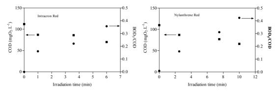
Figure 10.7: Evolution of BOD<sub>5</sub>/COD ratio and COD vs irradiation time for Intracron Red and Nylanthrene Red (100 mg.L<sup>-1</sup>).
