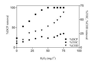
Figure 5.27: DCP, TOC and COD removal percentage as function of  $H_2 O_2$  in photo-Fenton process. [Fe (II)]<sub>i</sub>=10 mg. L<sup>-1</sup> experimental time 40 min.
