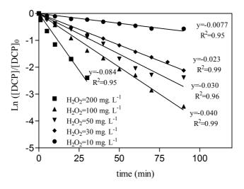
Figure 7.5: First order kinetic constant for DCP degradation by UV/H<sub>2</sub>O<sub>2</sub> photolysis
