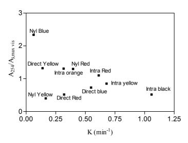
Figure 10.11 : Dye kinetic apparent constants versus specific absorbance at 254nm.
