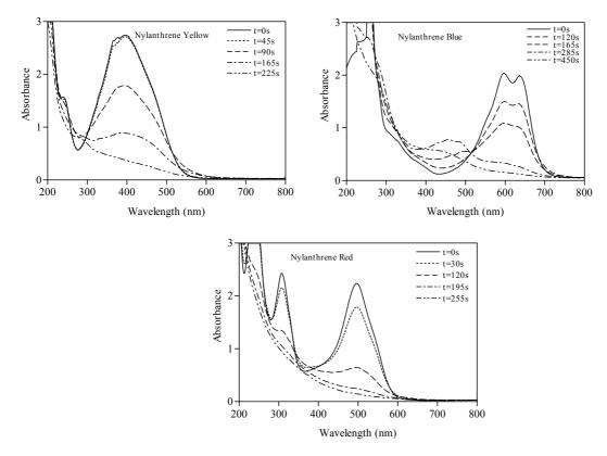
Figure 10.5 : VUV photolysis of Nylanthrene acid dyes (100 mg.L<sup>-1</sup>).
