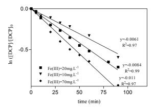
Figure 7.9: First order kinetic constant for DCP degradation by UV/Fe (III) process.
