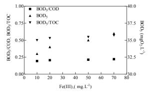
Figure 7.10: BOD<sub>5</sub>, BOD<sub>5</sub>/COD, BOD<sub>5</sub>/TOC evolution of POH treated solution as function of initial Fe(III) used in UV/Fe(III) process. Reaction time 90 min.
