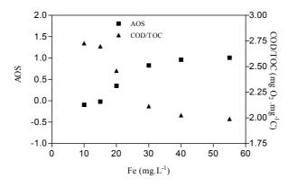
Figure 8.45: AOS and COD/TOC as function of initial Fe(II) in single lamp photo-reactor. $[H_2O_2]_i = 30$  mg.L<sup>-1</sup>, 50 min irradiation time and free pH evolution.
