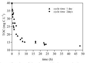
Figure 9.5: TOC evolution as function of time in aerobic SBR, cycle duration 1 and 2 days and feed  $BOD_5/COD=0.25$
