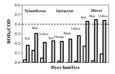
Figure 10.8: BOD<sub>5</sub>/COD evolution for initial and photolyzed dyes solutions (100 mg.L<sup>-1</sup>)
