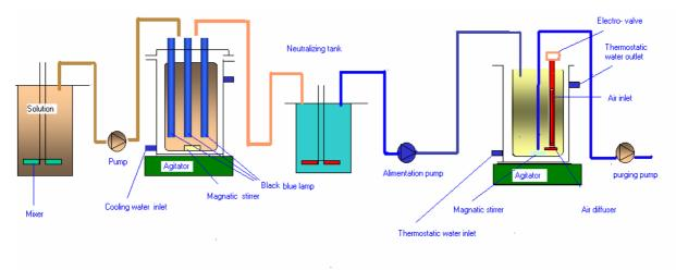
Figure 5.6: Photochemical-biological reactor installation
