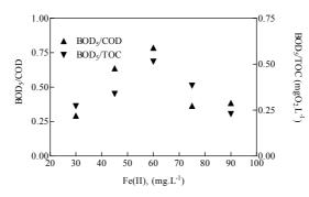
Figure 7.43: BOD<sub>5</sub>/COD and BOD<sub>5</sub>/TOC as function of initial Fe (II) concentration for photo-Fenton,  $[H_2O_2]_i = 300 \text{ mg-L}^{-1}$ , 40 min reaction time.
