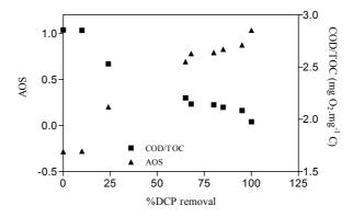
Figure 7.47: AOS and COD/TOC evolution as function of DCP removed. [Fe (II)]<sub>i</sub>= 10 mg.L<sup>-1</sup>,  $[H_2O_2]_i$ = 50, 40 min reaction time and free pH evolution .
