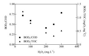
Figure: 7.39: BOD<sub>5</sub>/COD and BOD<sub>5</sub>/TOC as function of initial  $H_2O_2$  concentration for POH solution. [Fe (II)]<sub>i</sub>= 60 mg-L<sup>-1</sup>, 15 min reaction time.
