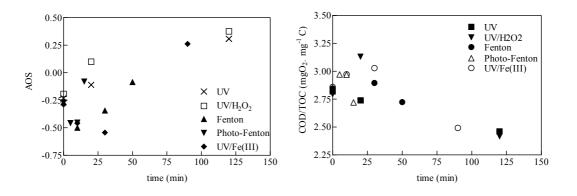
Figure 7.78: Change in oxidation state for the five processes during POH photo-degradation.  $[H_2O_2]_i = 30 \text{ mg.L}^{-1}$ ,  $[Fe(II)]_i = 10 \text{ mg.L}^{-1}$ ,  $[Fe(III)]_i = 70 \text{ mg.L}^{-1}$  and free pH evolution.
