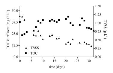
Figure 9.1: Total organic carbon evolution and TVSS as function of time during start up, feed  $BOD_5/COD=0.15$
