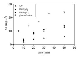
Figure 8.53: Dechlorination during different AOP's different AOP's. (A) single lamp photo-reactor, $[H_2O_2]_I = 50 \text{ mg.L}^{-1}$ ,  $[Fe(III)]_I = 70 \text{ mg.L}^{-1}$ ,  $[Fe(II)]_I = 10 \text{ mg.L}^{-1}$ , and free pH evolutions.
