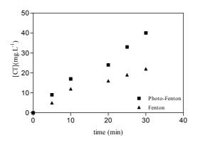
Figure 7.76: Dechlorination by Fenton and photo-Fenton process.  $[H_2O_2]_i = 50 \text{ mg.L}^{-1}$ ,  $[Fe(II)]_i = 10 \text{ mg.L}^{-1}$ ,  $[Fe(III)]_i = 70 \text{ mg.L}^{-1}$  and free pH evolution
