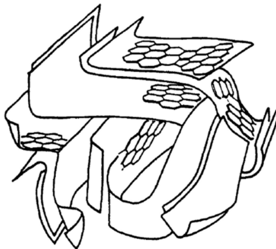
Figure 5 - Schematic of folded graphite-like layers [3]
