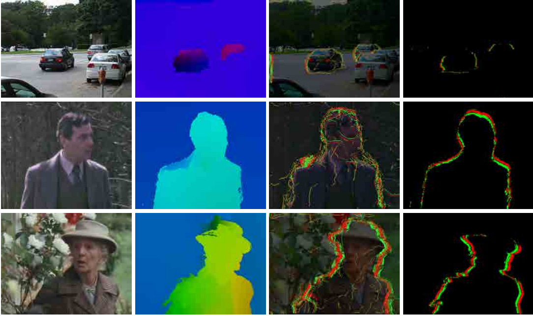
Figure 3.12: Three examples of occlusion detection. The left image shows the original frame, the center left image shows the modeled flows for a given partition. The two right images show the occlusion relations superposed to the image of the methods in Eq. (3.31) and Eq. (3.35). Occluded and disoccluded areas are shown in red, while their occluding pixel is shown in green. Note how the second method obtains clearer boundaries and much less false alarms.
