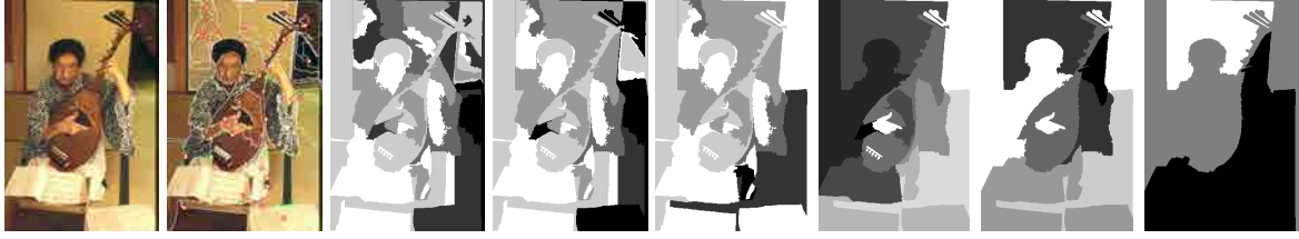
Figure 5.22: Examples of partitions obtained using tree cuts with the region cost (5.32). The first two images correspond to the original image and an oversegmentation showing the estimated T-junctions with the same color code as in Fig. 5.21. Partitions are obtained by increasing \lambda_o , so coarser partitions are obtained each time. Each region is colored with a different gray level.
