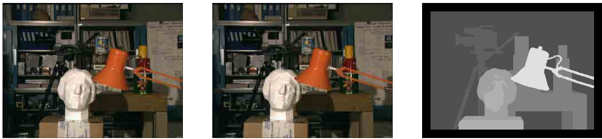
Figure 2.5: Depth perception from two views. From left to right: left image, right image and true depth map. The depth map can be constructed from binocular disparity.
