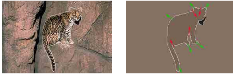
Figure 2.7: Example on how the minima rule is used to extract points of high curvature and a global depth decision from local convexity relations. In the left image the boundary of the animal is shown outlined in white. In the right, points with convexity are marked with green arrows, while points with red arrows indicate high concavity. The final depth decision results from averaging these points.
