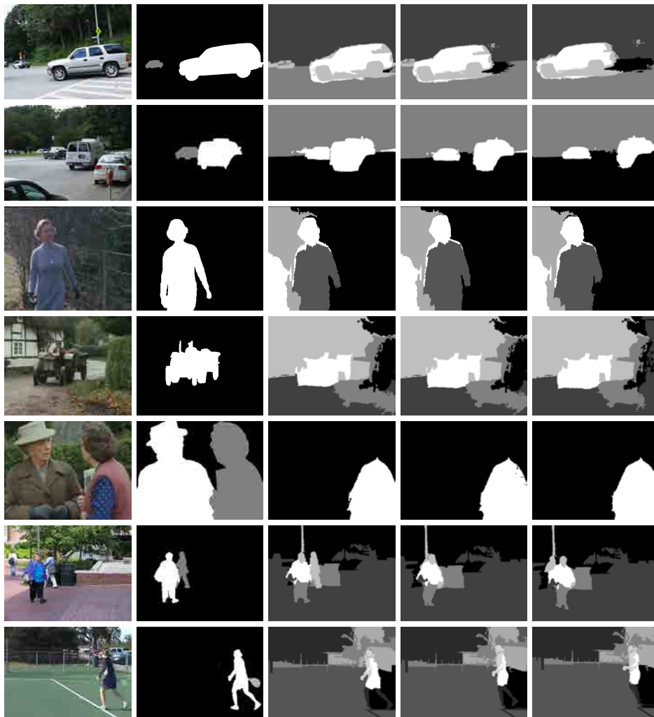
Figure 7.13: Examples of depth ordering in the MOSEG dataset. From left to right: reference frame, groundtruth depth ordering and results for first, sixth and tenth frame.
