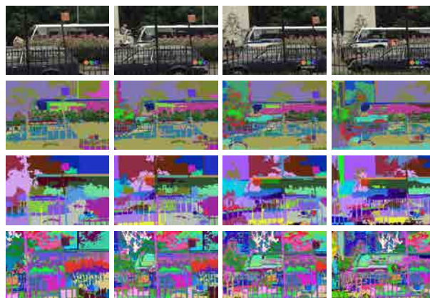
Figure 7.8: Video segmentation examples. Frames 1,11,21,31 from the bus sequence in the dataset (A. Y. C. Chen and Corso 2010). In row order, partitions obtained with the SWA method, the GBH algorithm and the proposed Trajectory BPT. Each region is colored with a unique color that is consistent over time. Each partition involves roughly 100 regions.
