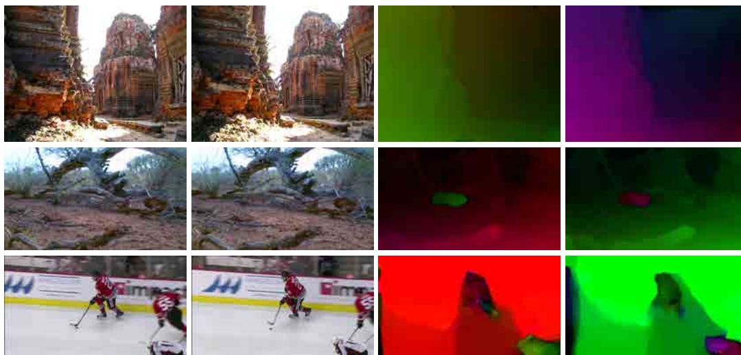
Figure 3.11: Optical flow estimation examples. The first column shows the frame at time t of the sequence and the second column shows frame at time t + 1 . The two last columns show the forward flow field (center right) and the backward flow field (right). Optical flow direction is color coded, whereas the flow magnitude is encoded in the color saturation.
