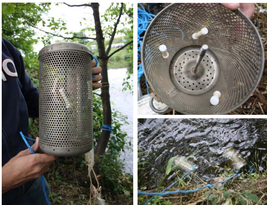
Figure 7 – Deployment of the ceramic dosimeter passive sampler in the River Aire (UK).
