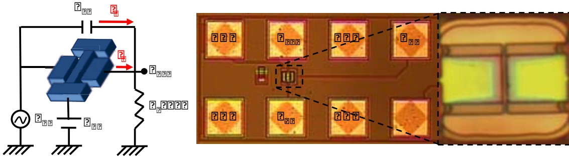
Figure 112.- Schematic electrical set-up for measuring stand-alone MEMS with capacitive transduction with a network analyzer. The optical image of a CCB with the output pads and zoom of the resonator are also depicted.
