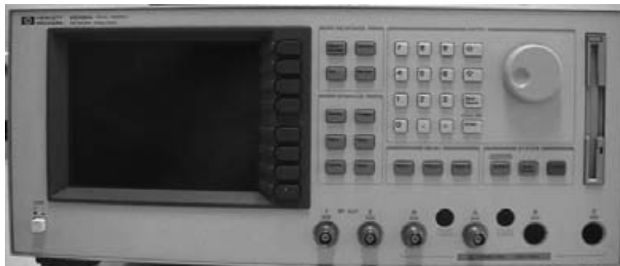
Figure 213.- Network analyzer E5100A from H&P (Agilent Technologies).
