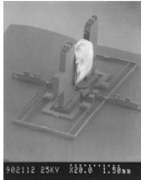
Figure 15.- Linear magnetic actuator with assembled coil [Guc98].
