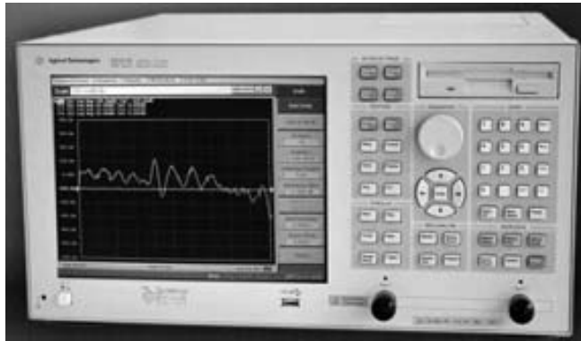
Figure 214.- Network analyzer E5071B from Agilent Technologies.
