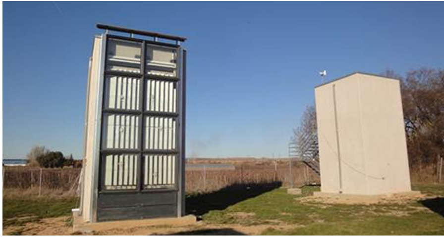
Fig. 2. Experimental set-up: reference and ventilated facade cubicles.
