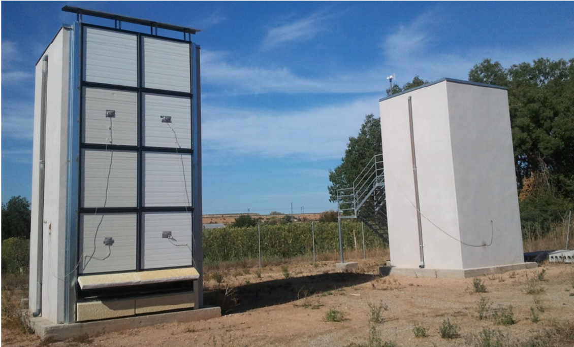
Figure 16. Experimental set-up: Ventiladed facade and reference cubicles during cooling season
