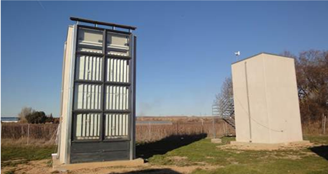
Figure 14. Experimental set-up: Ventiladed facade and reference cubicles during heating season
