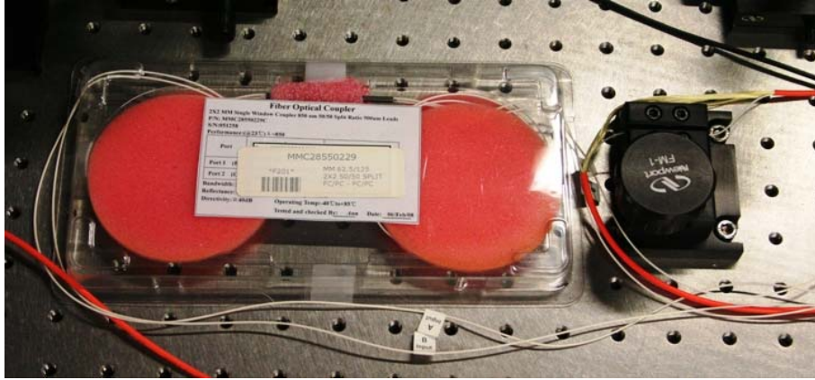
Fig. 50. 2x1 coupler and mode scrambler.
